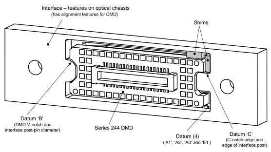
Figure 14. Alignment Shims
