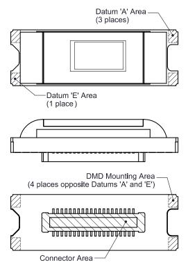
Figure 9. DMD Mechanical Loads
