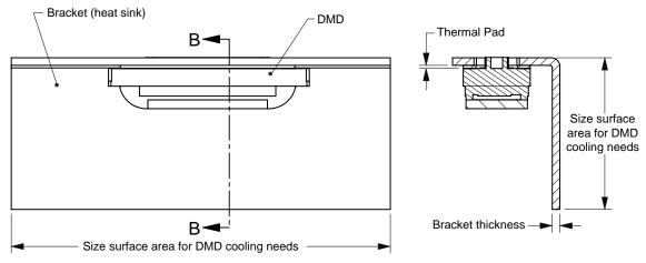
Figure 19. Mounting Bracket Thermal Considerations
