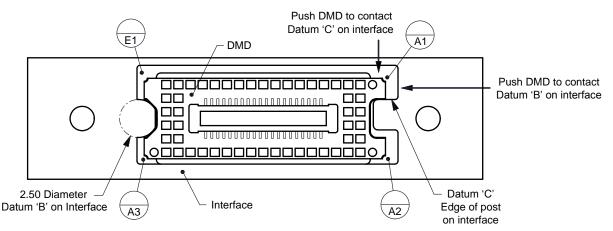
Figure 12. Mounting Datum 'B' Contact
