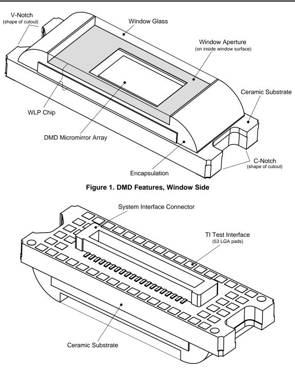
Figure 2. DMD Features, Electrical Side
