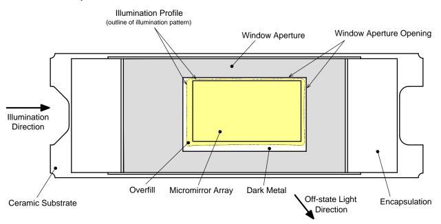
Figure 5. Optical Illumination Overfill
