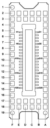
Figure 7. Pin Numbering Scheme
