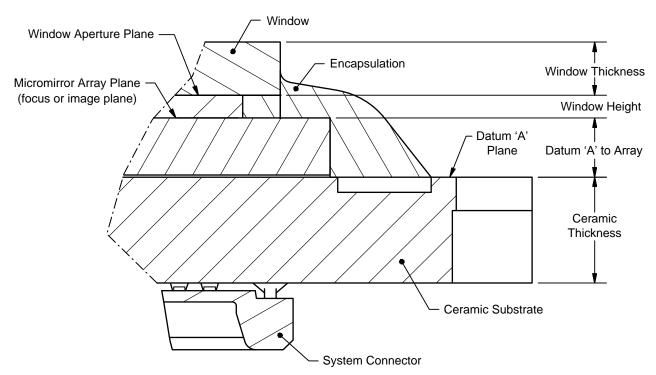
Figure 4. DMD Cross Section View Features
