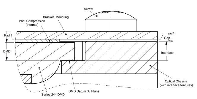
Figure 17. Gap Tolerance Analysis Schematic
