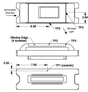
Figure 8. Thermal Test Points
