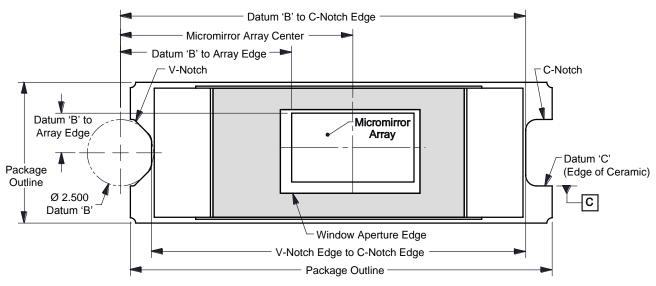
Figure 6. Micromirror Array Location
