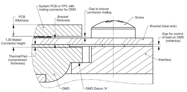
Figure 16. Critical Gap for Control of Load
