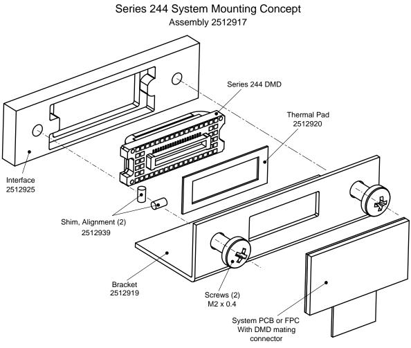
Figure 13. Shim Alignment System Mounting Concept
