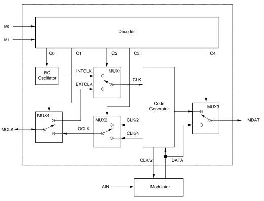
Figure 2. Flexible Interface Block Diagram
