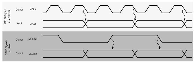
Figure 7. Input and Output Waveforms from CDI Circuit
