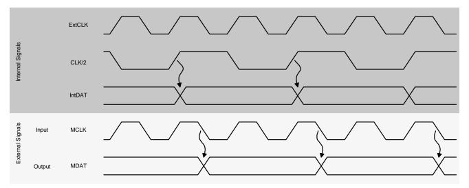
Figure 5. ADS1202 Output Waveform in Mode 3
