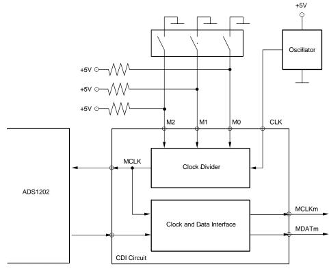
Figure 6. Structure of the CDI Circuit
