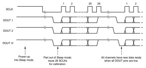
Figure 3. Power-Up Calibration Timing
