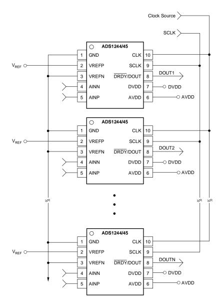
Figure 1. Standard Multi-Channel Configuration
