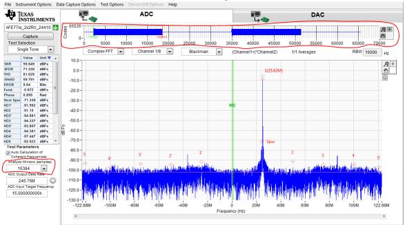
Figure 4-4. Spectrum of Receiver ADC in TDD Mode
