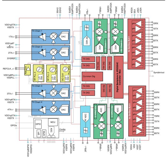
Figure 2-1. Block Diagram of the AFE77xx
