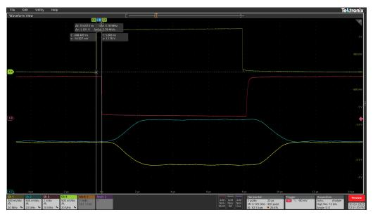
Figure 4. AMC23C11 Overvoltage Response Timing Waveform
