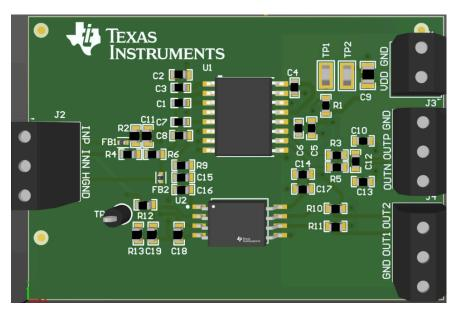
Figure 2. AMC3311 and AMC23C11 PCB Layout
