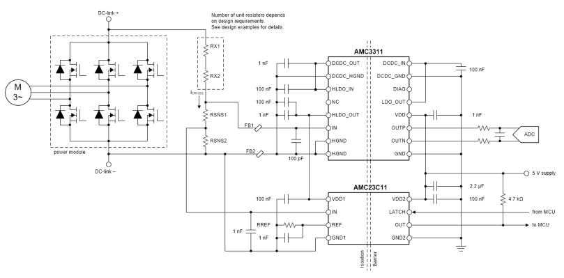
Figure 1. AMC3311 and AMC23C11 Schematic
