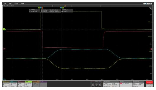
Figure 3. AMC3311 Overvoltage Response Timing Waveform
