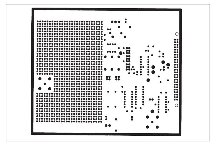
FIGURE 7. Bottom Soldermask of the DEM-ADS7812/13P Demonstration Board.
