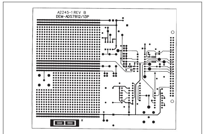
FIGURE 4. Component Side of the DEM-ADS7812/13P Demonstration Board.
