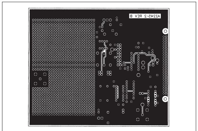
FIGURE 6. Ground Plane of the DEM-ADS7812/13P Demonstration Board.
