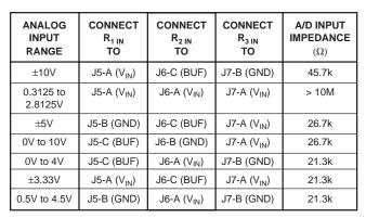
TABLE II. These are the Jumper Settings (J5, J6 and J7) for the Most Common Input Ranges to the ADS7812 and ADS7813. Note that all jumper configurations on the DEM-ADS7812/13P board are acceptable. Refer to Table IV of the ADS7812 or ADS7813 product data sheets for more details concerning other input range options. Configured for CIB testing.
