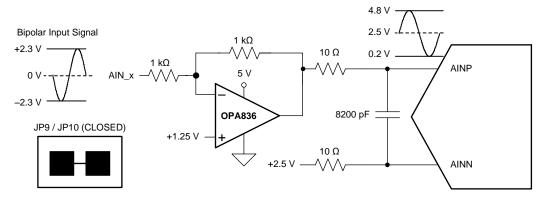
Figure 2. Bipolar Input Signal Configuration
