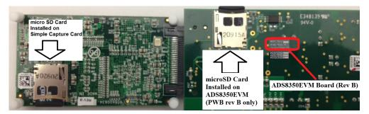
Figure 7. Bottom View of ADS8350EVM Rev B with microSD Card Installed
