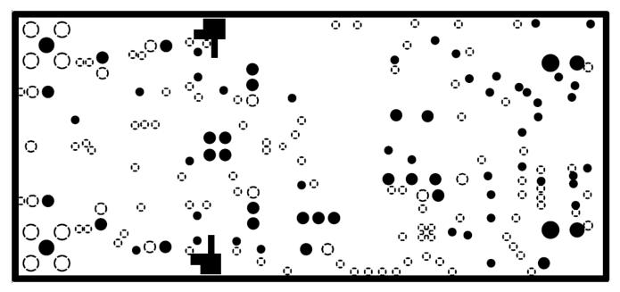
Figure 28. ADS8350EVM PCB: Ground Layer
