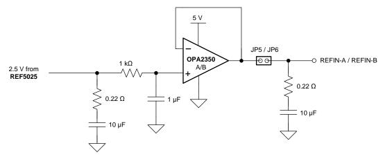
Figure 4. REFIN\_A and REFIN\_B Reference Connections
