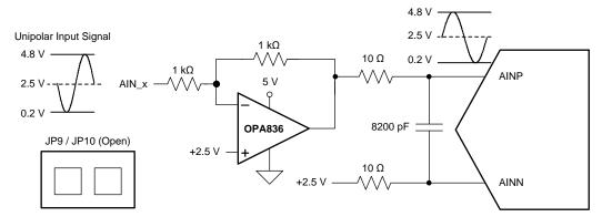
Figure 3. Unipolar Input Signal Configuration
