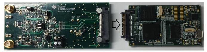
Figure 8. Connecting ADS8350EVM Board to Simple Capture Card Controller Board
