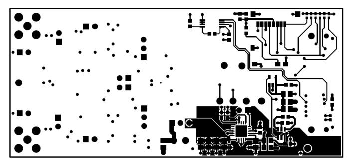
Figure 30. ADS8350EVM PCB: Bottom Layer
