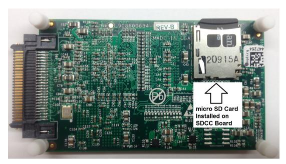
Figure 6. Bottom View of Simple Capture Card Board with microSD Memory Card Installed
