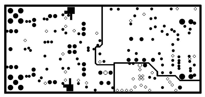
Figure 29. ADS8350EVM PCB: Power Layer
