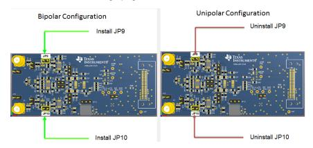
Figure 19. Bipolar or Unipolar Signal Jumper Settings Description on the GUI
