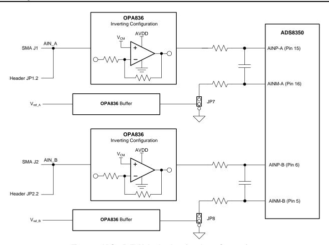
Figure 1. ADS8350EVM Analog Interface Input Connections
