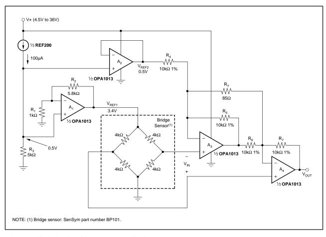
FIGURE 1. Single-Supply Bridge Measurement Circuit.
