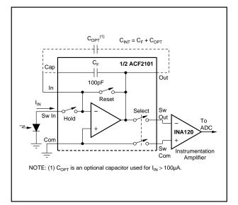
FIGURE 1. A Typical Application for the ACF2101 Switched Integrator.
