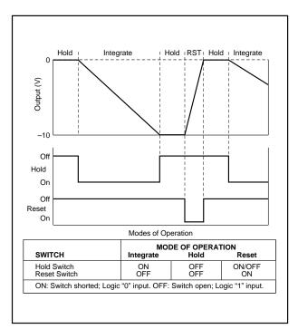
FIGURE 2. Modes of Operation for the ACF2101.
