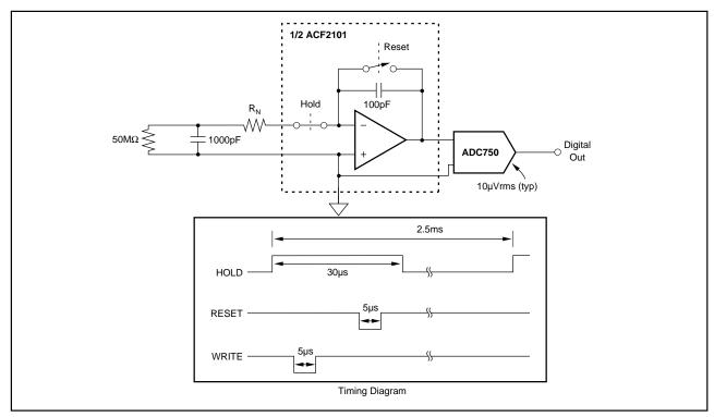
FIGURE 9. Circuit and Timing Diagram used to Test the Noise Performance of the ACF2101 with and without  $R_{\rm N}$ .
