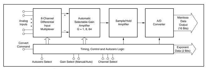
FIGURE 10. Block Diagram of ADC750 A/D Converter.
