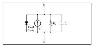
FIGURE 3. Photodiode Model Used in Noise Analysis.
