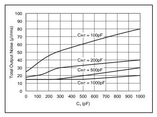
FIGURE 6. Total Output Noise of the ACF2101 Switched Integrator vs Parasitic Photodiode Capacitance,  $C_1$ , and the ACF2101 Integration Capacitor,  $C_{\rm INT}$ .
