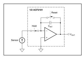
FIGURE 2. The ACF2101 Switched Integrator Block Diagram.
