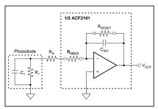
FIGURE 7. The ACF2101 Switched Integrator with an Additional Resistor, R<sub>N</sub>, Added in Series with the Photodiode to Reduce Noise.
