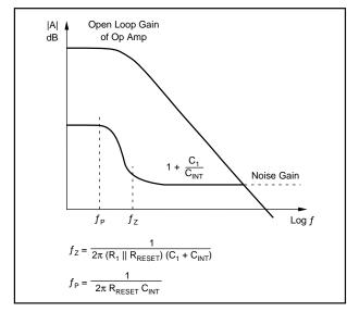
FIGURE 5. Noise Gain of the ACF2101, Switched Integrator.
