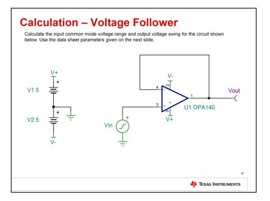
First, calculate the input common mode voltage range and output voltage swing for the circuit shown here, using the techniques and equations given in the input/output limitations lecture. Use the data sheet parameters given on the next slide.
