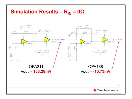
For the OPA211, you should get a result of around 133.28mV. For the OPA188, you should get a result of about -10.73mV.
