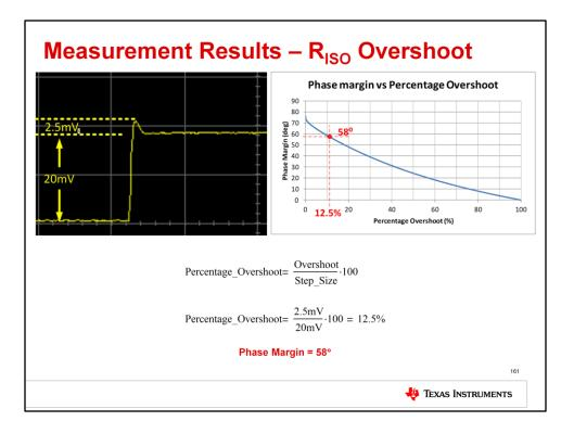
Use cursors to measure the amount of overshoot. You should see results similar to this. With Riso, the measured unloaded output overshoot was reduced to 12.5%, resulting in a phase margin of approximately 58 degrees which indicates a stable circuit.
