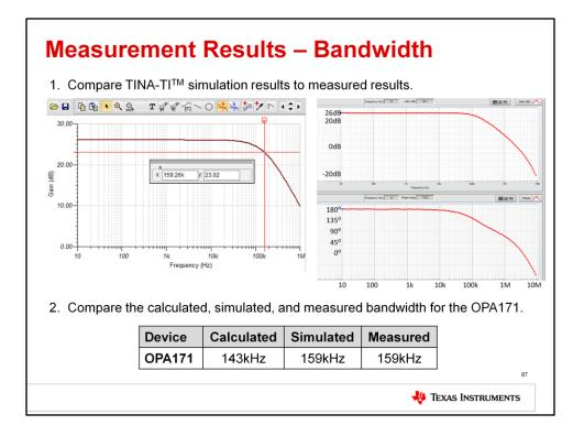
Compare the bandwidth measurement of the VirtualBench to the simulated results from TINA-TI. Compare this to your calculated results. You should see very good correlation between all three values, although your numbers may vary slightly.
