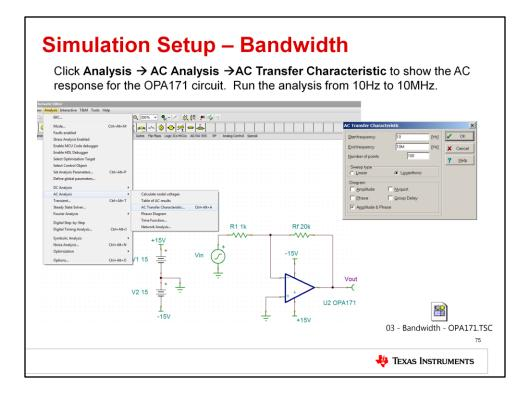
The next step is to run a SPICE simulation analysis for the AC transfer characteristic. This will allow us to see the op amp's closed loop bandwidth and DC gain in this configuration.
