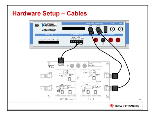
This slide gives the connection diagram between the TI Precision Labs test board and the National Instruments VirtualBench. Connect the provided power cable to the DC power supply of the Virtual Bench and power connector J4 on the test board. Connect Vout1 on the test board to VirtualBench oscilloscope channel 1, and Vout2 on the test board to Virtual Bench oscilloscope channel 2, using BNC cables.
