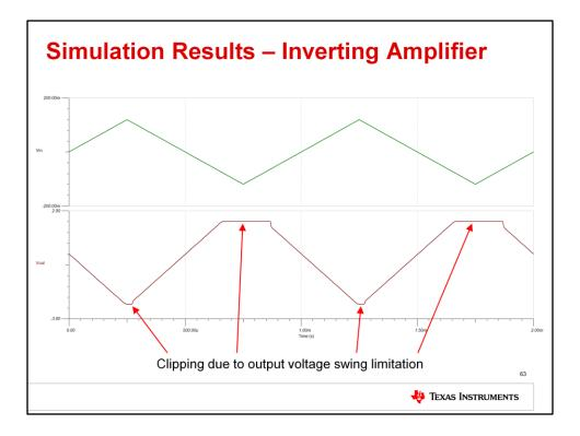
You should see a result similar to this. Vin is a triangle wave, as expected, but Vout clips at both the positive and negative ends of the triangle wave due to output voltage swing limitations.
