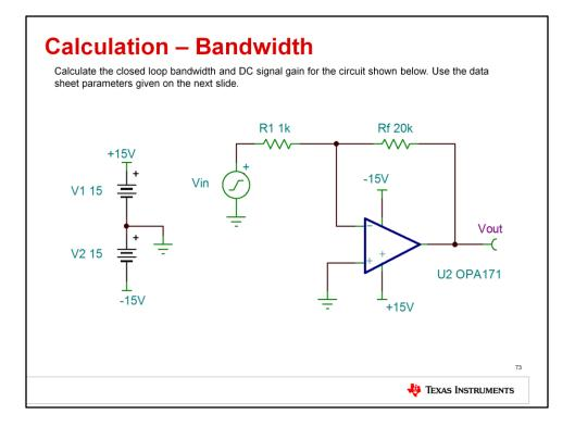
First, calculate the closed loop bandwidth and DC signal gain for the circuit shown here, using the techniques and equations given in the bandwidth lecture. Use the data sheet parameters given on the next slide.
