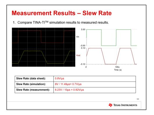
Compare the oscilloscope display of the VirtualBench to the simulation results from TINA-TI. Also compare the slew rate values from the data sheet, simulation, and measurement. They should all be similar, although you may get slightly different results.
