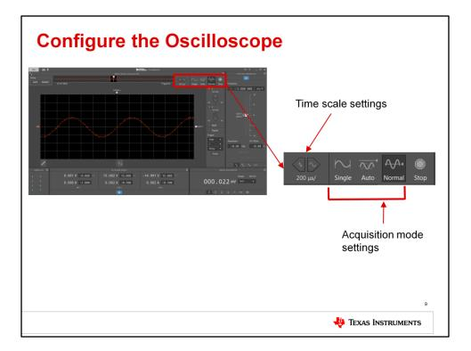
Here we set the horizontal time base on the scope as well as the triggering mode. "Auto" is untriggered roll or automatic triggering. Normal is triggered. For periodic signals it is best to use normal mode.
