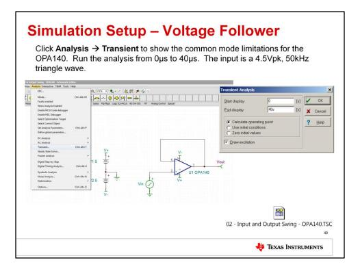
The next step is to run a SPICE simulation analysis for the transient output voltage behavior. This will allow us to see the op amp's output voltage response for a specified input signal, which in this case is a 2Vp, 1kHz triangle wave.
