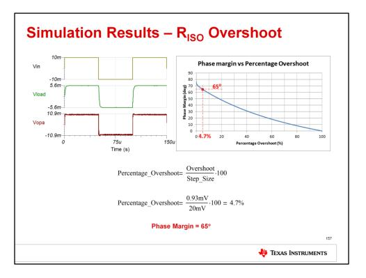
You should see results similar to this. With Riso added to the circuit, the overshoot was reduced to only 4.7%. This results in a phase margin of 65 degrees, indicating a stable circuit.
