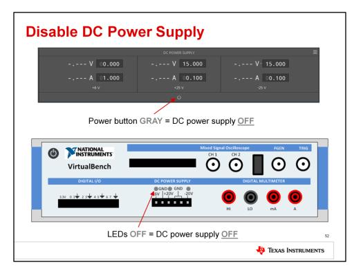
Make sure to disable the DC power supply before setting up the test PCB! In the VirtualBench software, click the power button in the DC Power Supply area to turn off the power. Check the front panel of the VirtualBench unit to make sure the LEDs are OFF!
