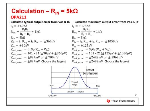
With RIN = 5k, the calculations change slightly since the voltage caused by IB is now affected by R\_IN. Use the new equation VIB =  $IB*R_EQ + IB*R_IN$ . Otherwise, the steps are the same as in experiment 1. Repeat the calculations for the maximum values.
