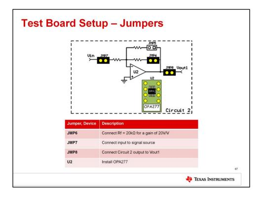
To prepare the test board for the measurement, install the jumpers and devices on circuit 2 as shown here.
