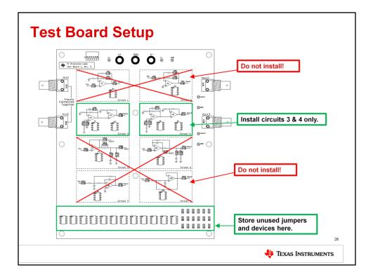
For the test board to function properly, it is important that you only install jumpers and devices in circuits 3 and 4. Do not install any jumpers or devices in any other circuits on the PCB! Remove any jumpers or devices from the unused circuits and store them in the storage area at the bottom of the test board.
