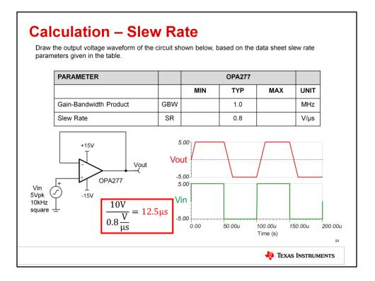
First, draw the output voltage waveform of the circuit shown below. Use the slew rate specifications given in the table and the techniques from the slew rate lecture.
