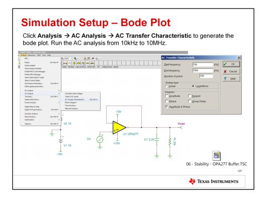
Next, run a SPICE simulation analysis for the AC transfer characteristic. This will allow us to see the op amp's AC peaking, which is another indicator of phase margin.
