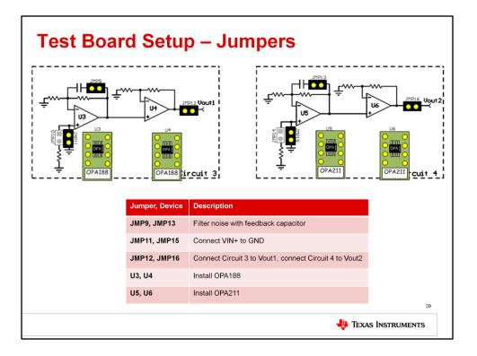
To prepare the test board for the measurement, install the jumpers and devices on circuit 3 and circuit 4 as shown here.
