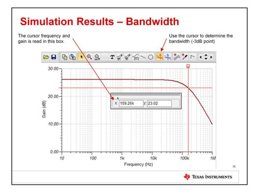
You should see a result similar to this. Enable the cursor, then check the DC gain, or gain at minimum frequency. The result will be 26dB, or 20V/V. Next, find the -3dB point, or the frequency where gain drops to 23dB. This occurs at 159kHz.
