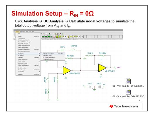
The next step is to run a SPICE simulation analysis for the total DC output voltage. The necessary TINA-TI simulation schematics are embedded in this slide set – simply double-click the icons to open them. Ensure that the jumpers are set correctly. In the OPA211 circuit, JMP13 and JMP14 are open, and JMP15 is closed. In the OPA188 circuit, JMP9 and JMP10 are open, and JMP11 is closed.
