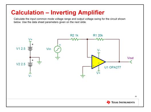
First, calculate the input common mode voltage range and output voltage swing for this inverting amplifier circuit, using the techniques and equations given in the input/output limitations lecture. Use the data sheet parameters given on the next slide.
