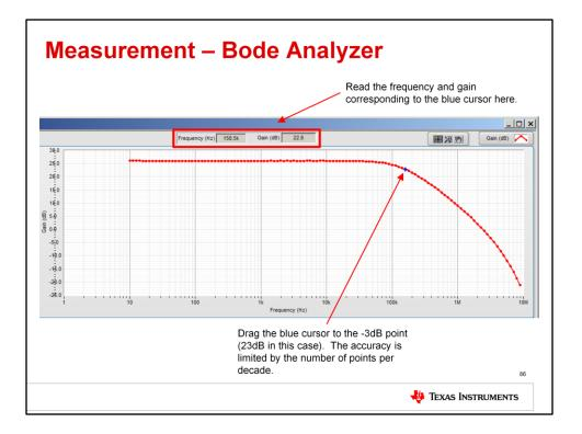
You should see a result similar to this. Enable the cursor, then drag the cursor to the - 3dB point, or 23dB in this case. Take note of the frequency – in this case the result is 159kHz, although your results may vary slightly.
