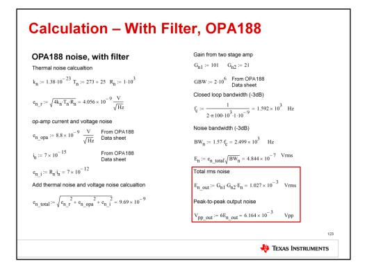
The steps in the calculation are nearly the same as before. However, this time the filter capacitor must be taken into account when calculating the circuit's closed-loop bandwidth. With the filter capacitor connected, the closed-loop bandwidth is computed to be 1.59kHz. Without the capacitor, the bandwidth was 19.8kHz! As expected, this helps to reduce the total noise.
