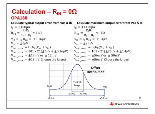
Repeat the same procedure for the OPA188. The different specifications of the OPA188 will give a different output voltage result in both the typical and maximum case.
