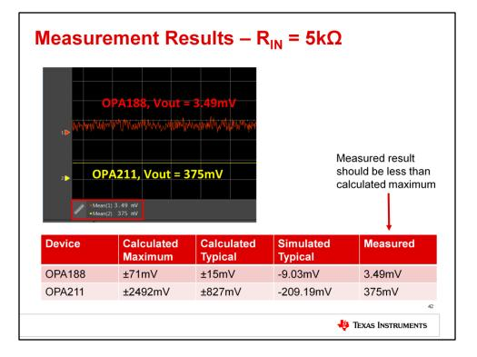
In experiment 2, the OPA188 has a measured output voltage of 3.49mV, and the OPA211 has a measured output voltage of 375mV. You may have different results in your experiment.
