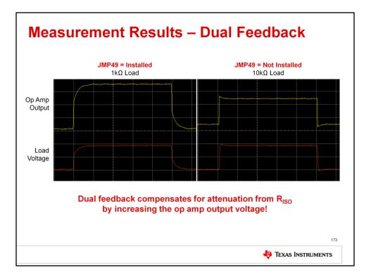
You should see results similar to this. As you can see, the load voltage remains accurate, even with changing load, due to the compensation provided by the dual-feedback network. The unloaded op-amp output voltage must increase as the load resistance decreases to minimize the output voltage divider effect.
