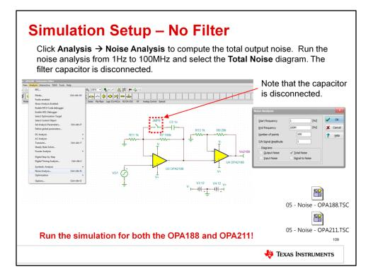
The next step is to run a SPICE simulation analysis for the total output noise. Simply open the TINA-TI simulation schematics embedded in the presentation, ensure that filter capacitor jumper is open, then select Analysis, followed by Noise Analysis. Make sure that "total noise" is selected, then run the analysis from 1Hz to 100MHz.
