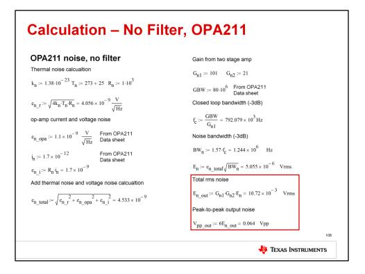
This slide shows the calculation for the OPA211. The op amp's input voltage and current spectral density, as well as the op amp gain bandwidth product, are different, but the steps of the calculation are exactly the same. Simply substitute in the new values and take note of the result.
