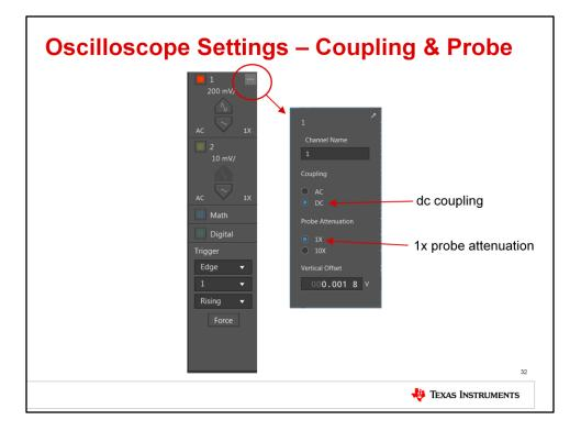
The icon at the top right of the oscilloscope opens a new window with more options for each channel. Each channel can be given a custom name. Set the coupling mode to dc. Set probe attenuation to 1x.
