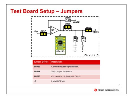
To prepare the test board for the measurement, install the jumpers and devices on circuit 5 as shown here.
