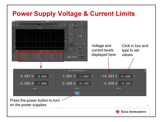
This slide shows the location of power supply voltage and current settings. Also, the button in the center turns on and off the supplies.
