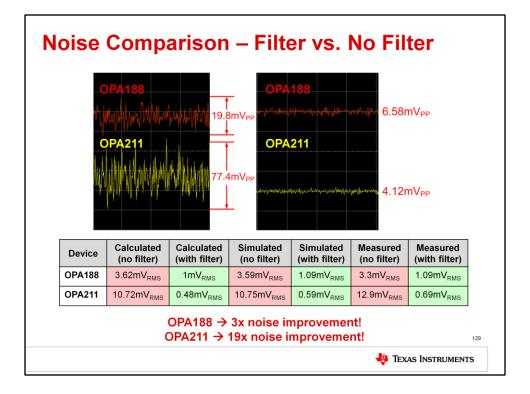
This slide compares the noise performance of both the OPA188 and OPA211, with and without the filter. It should be clear just from the oscilloscope capture that the filter gave us a massive improvement in noise. If you compare the peak-to-peak noise values in the table, you can see that with the filter, we achieved a 3x improvement with the OPA188 and a 19x improvement with the OPA211!
