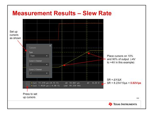
Let's now determine the measured slew rate. Enable cursors, set them up as shown, then place the cursors on 10% and 90% of the output signal. Take note of the time and voltage difference, and then calculate the slew rate using the equation given. In this example, a slew rate of 0.82V/us was measured. You may have different results in your experiment.
