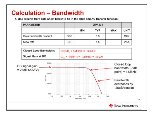
This circuit uses the OPA171. In order to perform the calculations, you need to know the gain bandwidth product and for that device. That value is given here.
