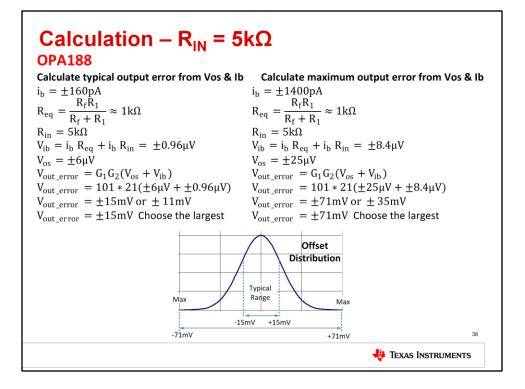
Repeat both sets of calculations for the OPA188, again using typical and maximum values. As before, the different electrical characteristics of the OPA188 will result in different output voltage calculations.
