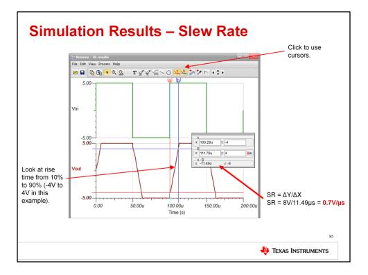
You should see a result similar to this. Vin is a square wave, as expected, but Vout must obey the slew rate limitations of the OPA277. You can see this effect in the rise time from 10% to 90% of the output, or -4V to 4V. Use the cursors to measure the time required to slew from -4V to 4V, and use the equation that slew rate = delta y over delta x to calculate the simulated slew rate of  $0.7V/\mu s$ .
