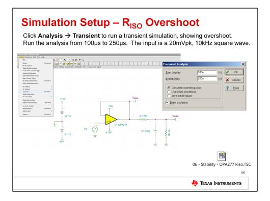
Let's now simulate the transient overshoot with Riso included in the circuit. As before, click Analysis  $\rightarrow$  Transient to run the simulation. Run the analysis from 0ms to 150us. The input is a 20mVpk, 10kHz square wave.
