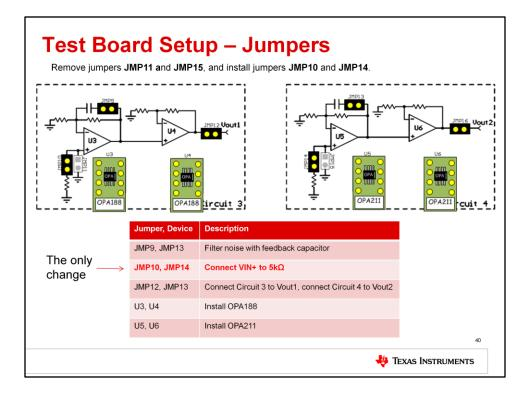
The jumper settings on the test board must be modified before re-running the bench measurement. Remove jumpers JMP11 and JMP15, and install jumpers JMP10 and JMP14. All other jumpers and devices remain the same from the previous experiment.
