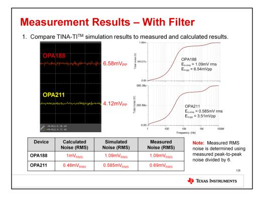
The expected output voltage noise results from the measurement with the filter are shown here. The OPA188 has a measured noise of 6.58mVpp, or 1.09mVrms, and the OPA211 has a measured noise of 4.12mVpp, or 0.69mVrms. Like before, the calculated, simulated, and measured results all match quite closely. The real question is: how much benefit did we get by adding the filter capacitor?
