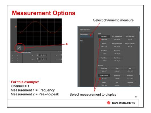
The VirtualBench can also make measurements automatically. Click the ruler icon, above the digital I/O settings, to open the measurement options window. Here you can select what channel to measure, and which measurement you want to display.
