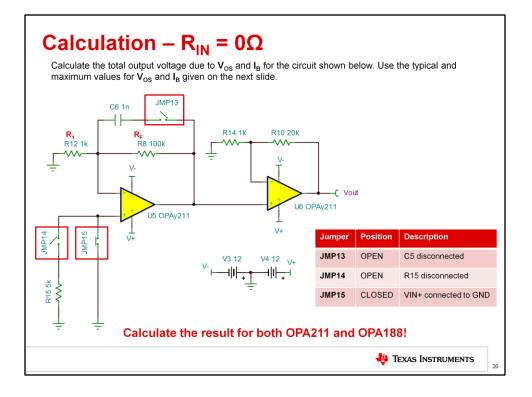
First, calculate the expected total output voltage due to VOS and IB for the circuit shown here, using the techniques and equations given in the VOS and IB lecture. Take note of the jumper positions in the table. JMP13 and JMP14 are open, and JMP15 is closed. JMP15 shorts the non-inverting input of U5 to ground, causing RIN to be 0 ohms.
