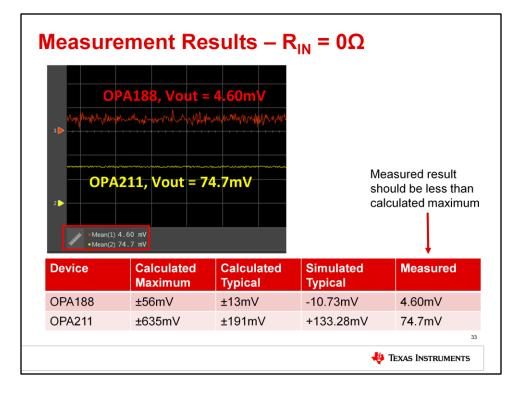
The expected output voltage results from the measurement are shown here. The OPA211 has a measured output voltage of 74.7mV, and the OPA188 has a measured output voltage of 4.60mV. You may have different results in your experiment.
