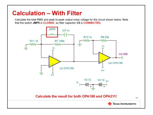
Perform another total noise calculation on the circuit shown. However, this time a filter capacitor is added to the feedback network of the first amplifier stage. This capacitor will reduce the circuit's noise bandwidth, so the overall noise performance will be significantly improved. As before, do the calculations with both the OPA188 and OPA211.
