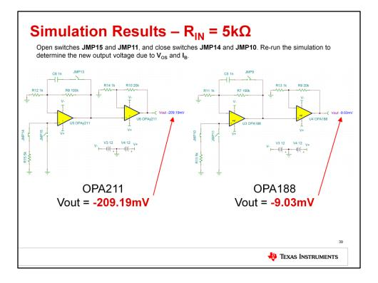
Re-run the simulated DC nodal voltage analysis, making sure to use the proper jumper settings.
