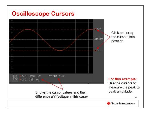
The cursors location may be adjusted to make a measurement. Click and drag the cursor indicators into position at the top and bottom of the sinusoidal waveform. The voltage level at each cursor, as well as the delta Y, in this case voltage difference, will be displayed next to the cursor icon. Use the cursors to measure the signal's peak-to-peak amplitude.
