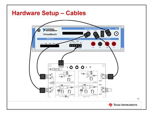
This slide gives the connection diagram between the TI Precision Labs test board and the National Instruments VirtualBench. Connect the provided power cable to the DC power supply of the Virtual Bench and power connector J4 on the test board. Connect Vin2 on the test board to VirtualBench channel FGEN, or function generator. Then connect Vin1 on the test board to VirtualBench oscilloscope channel 1, and Vout1 on the test board to VirtualBench oscilloscope channel 2.
