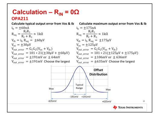
One important point to note is that IB and VOS can be positive or negative. This means that there are different possibilities for the output voltage due to VOS and IB which must all be considered.
