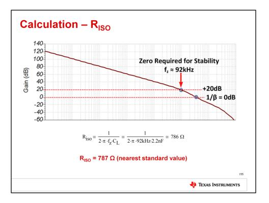
For best results, Riso should create a zero in the loop response 20dB greater than the frequency where the open-loop gain intersects with the closed-loop gain. This circuit is a buffer with a closed-loop gain of 0dB, so the zero should occur at 20dB. The open-loop gain is equal to 20dB at 92kHz. Use this value and the load capacitance to calculate Riso, which is 786 ohms in this example. 787 ohms is the nearest standard value resistance.
