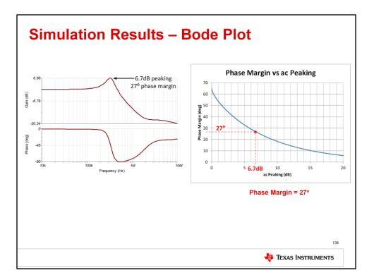
You should see a result similar to this. The 9dB of simulated AC peaking results in a phase margin of approximately 20 degrees.
