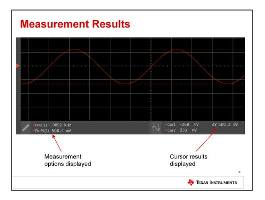
The measurement results are displayed next to the ruler icon. You should read a result of 1kHz, 500mVpp – the same as the function generator. The amplitude should be the same as the delta Y measurement from the cursor.
