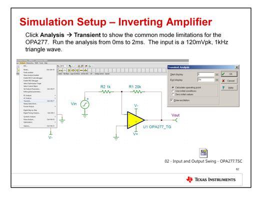
Run a SPICE simulation as before, but now using this inverting amplifier circuit with the OPA277.
