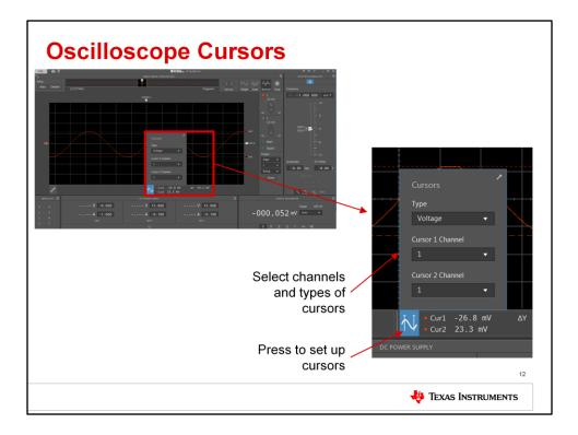
Cursors may be used to measured oscilloscope signals. Click the cursor icon, located above the power supply settings, to open the cursor menu. Select voltage type, then select the channel for the cursors.
