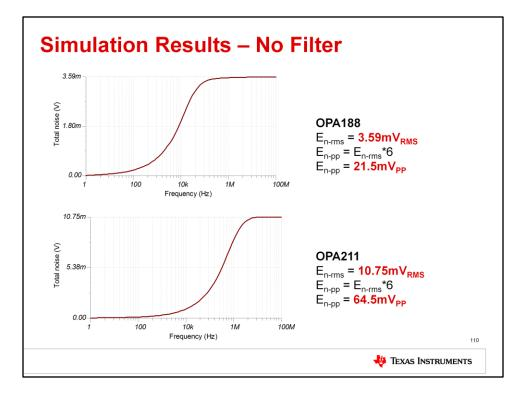
Over the 100MHz frequency range, the OPA188 circuit has a total noise of 3.59mVrms, or 21.5mVpp. The OPA211 circuit has a total noise of 10.75mVrms, or 64.5mVpp.
