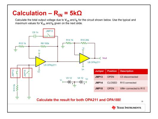
As shown in the schematic, jumper JMP15 shorting the positive input of U5 to ground is now removed. Jumper JMP14 is now installed in order to connect the positive input of U5 to a 5k $\Omega$  resistor. The IB of U5 will now flow through this resistor, developing a DC voltage due to Ohm's law and increasing the amount of offset voltage.
