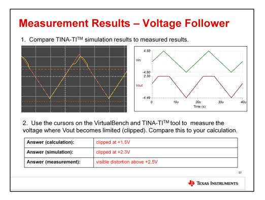
The expected measurement results are shown here. Compare the oscilloscope display of the VirtualBench to the simulation results from TINA-TI. Also, use the cursors on the VirtualBench and TINA-TI tool to measure the voltage where Vout becomes limited, or clipped. Compare this to your calculation.
