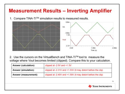
Compare the TINA simulation results to your measured results. The shape of the output waveform should look very similar, with hard clipping at the top of the waveform. Your device may or may not clip at the bottom of the waveform.
