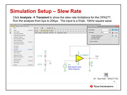
The next step is to run a SPICE simulation analysis for the transient output voltage behavior. This will allow us to see the op amp's output voltage response for a specified input signal, which in this case is a 5Vp, 10kHz square wave.
