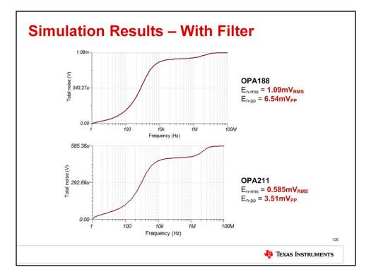
With the filter capacitor connected, the OPA188 circuit has a total noise of 1.09mVrms, or 6.54mVpp. The OPA211 circuit has a total noise of 0.585mVrms, or 3.51mVpp.
