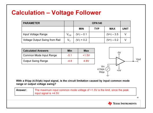
This circuit uses the OPA140. In order to perform the calculations, you need to know the input voltage range and voltage output swing values for that device. Those values are given here.
