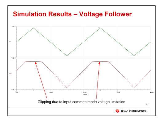
You should see a result similar to this. Vin is a triangle wave, as expected, but Vout cannot exceed +1V. This is due to the input common mode voltage limitation of the OPA735.
