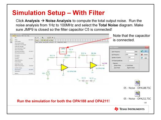
Run another SPICE simulation analysis for the total output noise. This time, ensure that the filter capacitor jumper is closed so that the capacitor is connected! As before, select Analysis, followed by Noise Analysis. Make sure that "total noise" is selected, then run the analysis from 1Hz to 100MHz.
