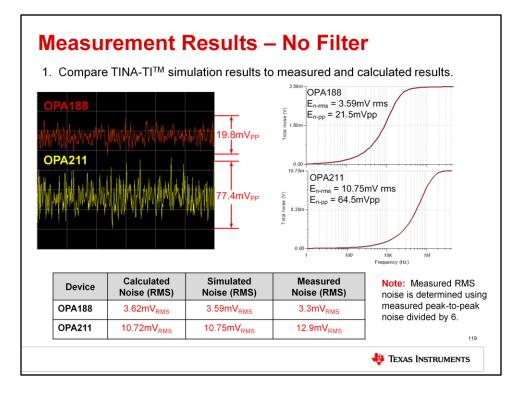
The expected output voltage noise results from the measurement are shown in the screenshot at the top left. The OPA188 has a measured noise of 19.8mVpp, or 3.3mVrms, and the OPA211 has a measured noise of 77.4mVpp, or 12.9mVrms. As you can see from the table, this agrees extremely well with the results from calculation and simulation!
