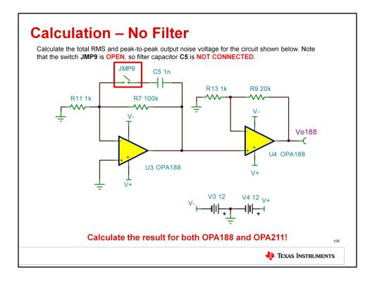
First, calculate the expected total RMS and peak-to-peak output noise voltage for the circuit shown here, using the techniques and equations given in the noise lecture. Note that the switch **JMP9** is open, so filter capacitor C5 is not connected to the circuit. Make this calculation twice – first with the OPA188 selected for U1 and U2, then with the OPA211. The different parameters of these op amps will give you different noise results.
