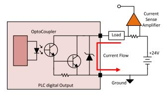
Figure 2. PLC Digital Output Sinking Current Circuit
