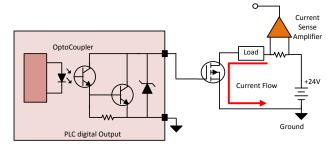
Figure 3. PLC Discrete Digital Output Control
