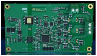
Figure 4. TI Design TIDA-01418 Circuit Board
