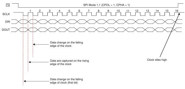
Figure 37. Clock Phase and Polarity: Mode 11
