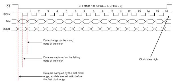
Figure 36. Clock Phase and Polarity: Mode 10
