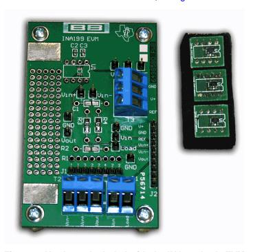
Figure 1. Hardware Included with the INA199A1-A3EVM
