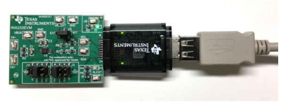
Figure 3-5. INA233 Power Up Using SM\_USB DIG and INA233EVM GUI Software
