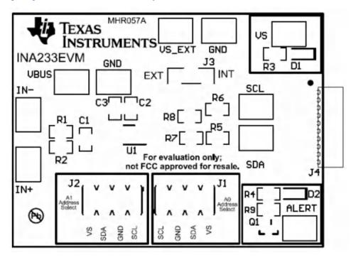
Figure 5-2. INA233EVM PCB Top Overlay
