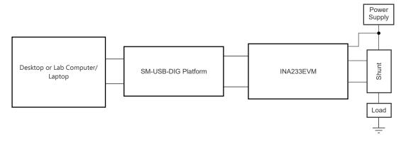
Figure 2-1. INA233EVM Hardware Setup
