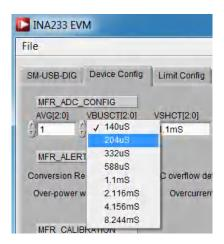
Figure 4-5. Configuring Conversion Times
