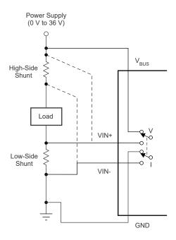
Figure 3-7. INA233 Shunt Configurations
