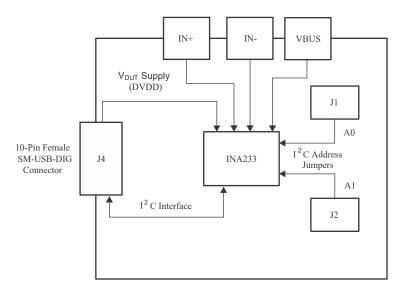
Figure 2-2. INA233EVM Board Block Diagram
