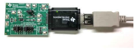
Figure 3-4. Connecting the INA233 Test Board and SM-USB-DIG Platform Board
