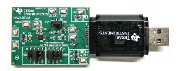
Figure 3-3. Connecting the INA233 Test Board and SM-USB-DIG Platform Board to the Computer
