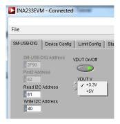
Figure 4-3. Setting the I<sup>2</sup>C Address
