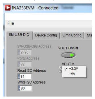
Figure 3-6. VDUT Voltage Selection in INA233EVM GUI
