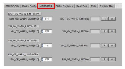
Figure 4-10. Set the Warning Limit Registers
