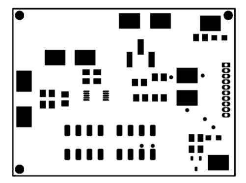
Figure 5-3. INA233EVM PCB Top Solder
