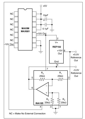
FIGURE 4. ±5.0V Reference Using REF102 Can Operate on Single +5V Power Supply.
