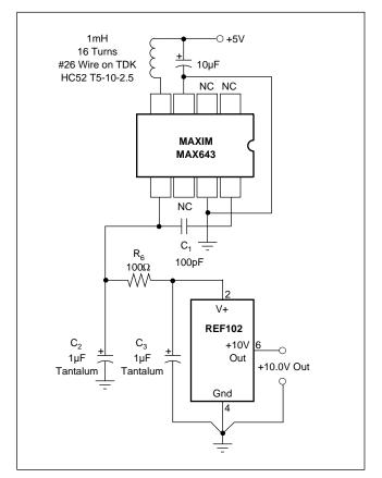
FIGURE 3. +10.0V Reference Using REF102 Can Operate on Single +5V Power Supply.
