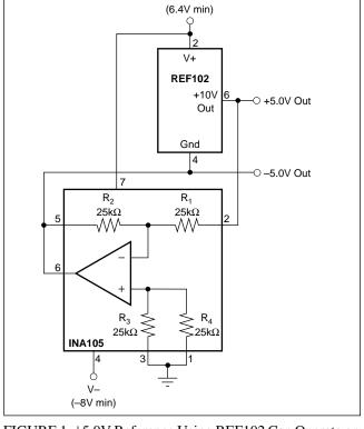
FIGURE 1.  $\pm 5.0V$  Reference Using REF102 Can Operate on +V<sub>s</sub> = +6.4V, -V<sub>s</sub> = -8V.
