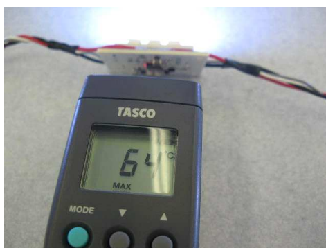
Figure 32. TLC5970 Reference Design Module Temperature Measurement: I_{LED} = 20 mA Each
