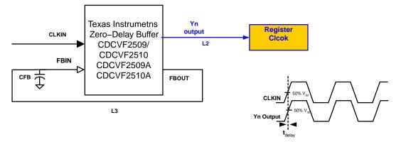
Figure 1. L2=L3, Zero Phase Delay Between CLKIN and Yn
