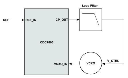
Figure 1. CDC7005 With Loop Filter and VCXO
