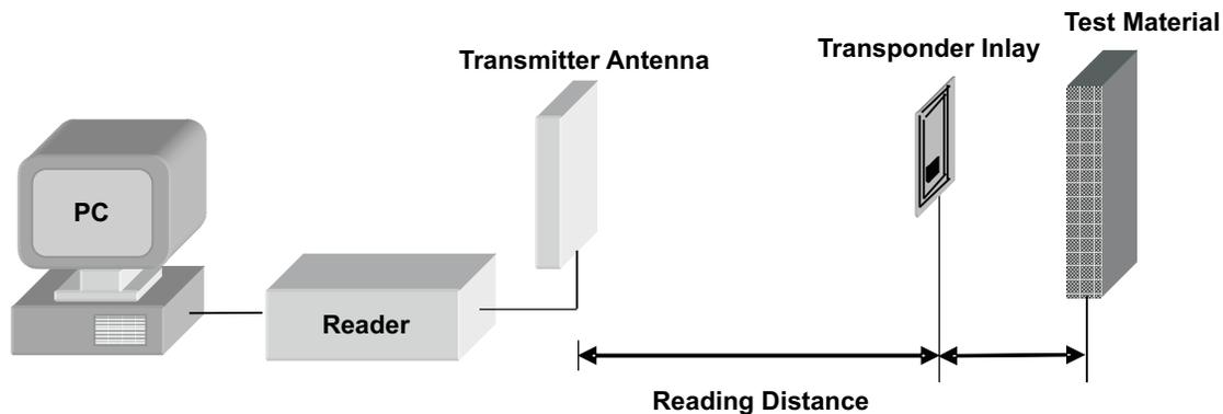
Figure 2-1. Test Set-up
