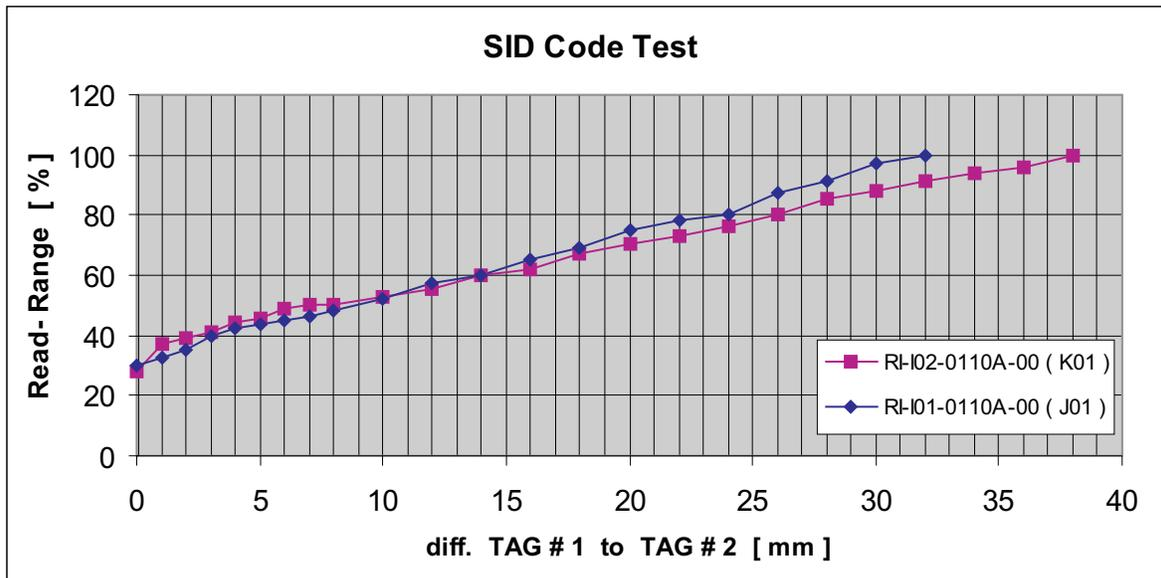
Figure 3-3. Effects of a Second Transponder Inlay
