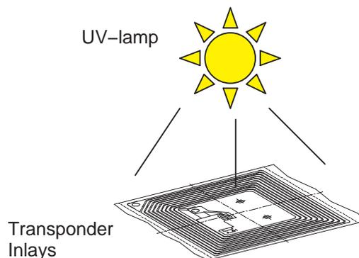
Figure 3-4. UV-Sensitivity Test Set-up
