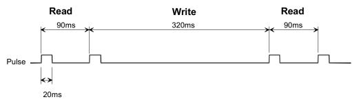
Figure 5. Timing Pulses From a Master Controller
