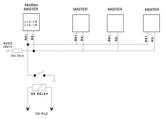
Figure 4. PLC Operated Timing Bus
