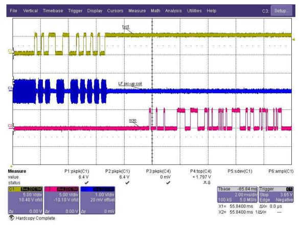
Figure 15. Complete Transponder Communication
