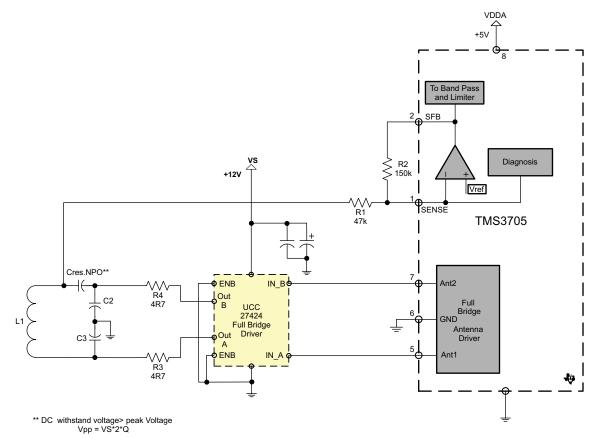
Figure 2. TMS3705x With External Amplifier
