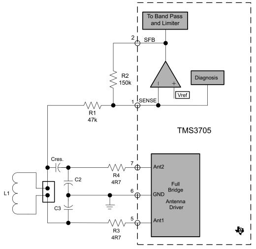
Figure 1. Standard HDX RFID Reader Configuration
