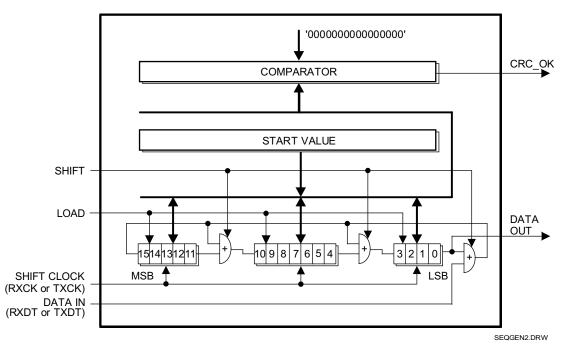
Figure 16. Block Schematic of CRC Generator
