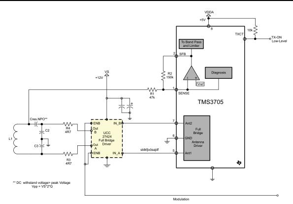
Figure 10. Schematic Connection of the Driver IC (UCC27424)
