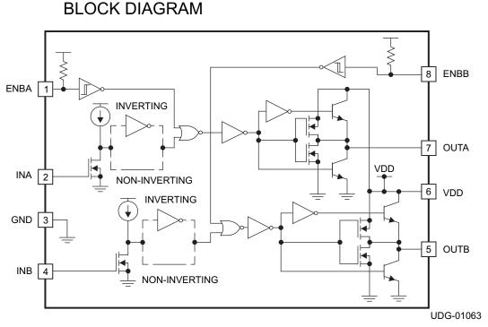
Figure 3. Circuit Block Diagram of External Amplifier UCC27424
