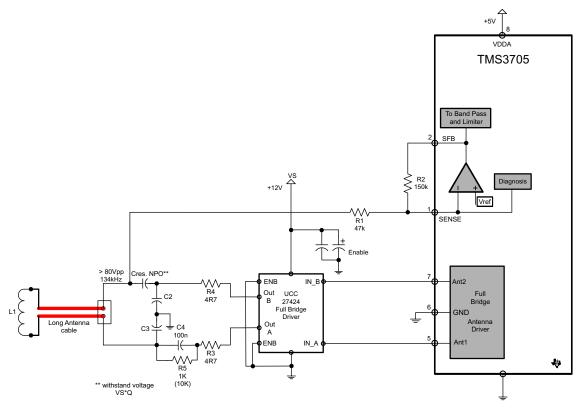
Figure 6. Extended Power Configuration with "Long" Antenna Cable
