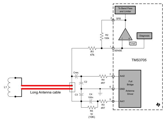
Figure 5. Conventional "Long" Antenna Cable Solution
