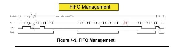
**Note:** As long as DOUT is at level 1 it is not permitted to send a clock signal on the SCLOCK line.
