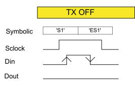
Figure 4-3. Shut Down Command
