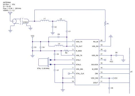
Figure A-1. Application Circuit
