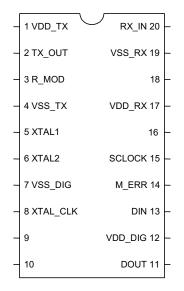
Figure 2-2. Transceiver Pins
