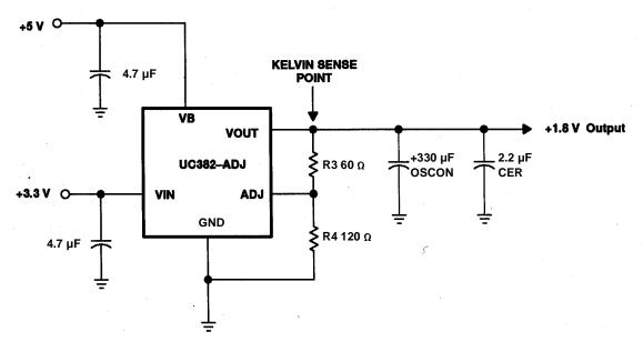
Figure 16. Kelvin-Sensing Circuit
