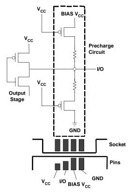
Figure 15. Typical BIAS V<sub>CC</sub> Connection Sequence
