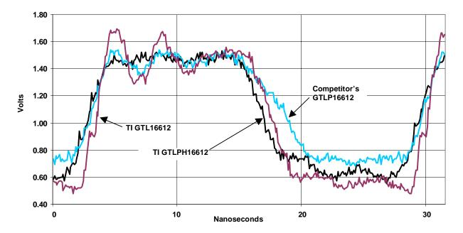
Figure 4. Demonstration of Output Edge Control
