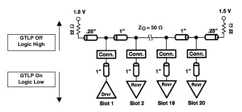
Figure 5. GTLP Open-Drain Backplane Physical Representation
