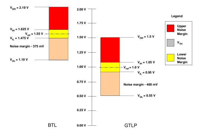
Figure 17. Comparison of BTL to GTLP Signal Levels
