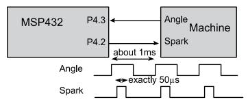
The input, **Angle**, is a periodic signal with a frequency of 20 to 1000 Hz (has a period of 1 to 50 ms). The output, **Spark**, should be a positive pulse (exactly 50  $\mu$ s wide) every time **Angle** goes from 0 to 1. The delay between the rising edge of **Angle** and the start of the **Spark** pulse should be as short as possible. The period of **Angle** can vary from 1 ms to 50 ms. Since **Angle** is an input you cannot control it, only respond to its rising edge.
