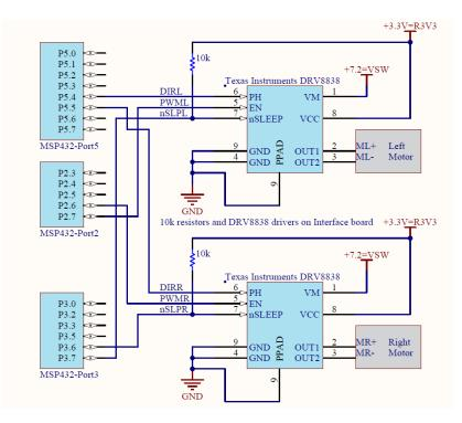
Figure 1. Interface circuit.
