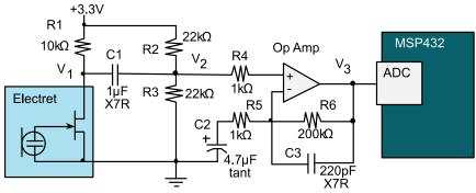
Figure 5B. Second possible microphone input circuit (option B).
