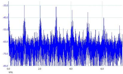
Figure 8A. Frequency spectrum of the output of the distance sensor (without analog filter).
