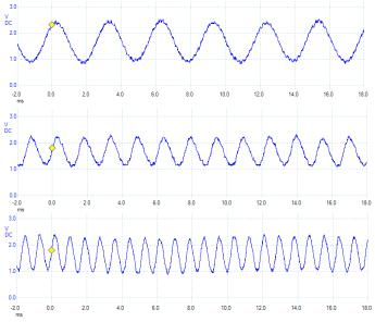
Figure 3B. Typical outputs of the microphone circuit (option B).
