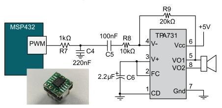
Figure 4B. One possible speaker output circuit (option B).
