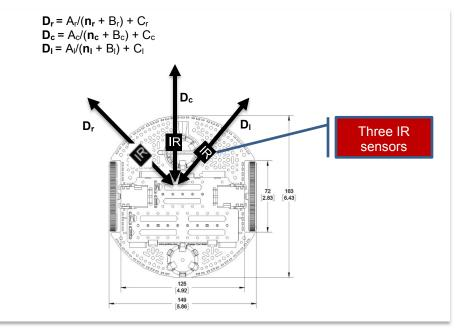
Figure 3A. Distance defined from a central point on the robot (option B).
