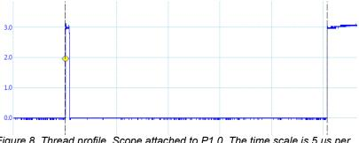
Figure 8. Thread profile. Scope attached to P1.0. The time scale is 5  $\mu s$  per division.
