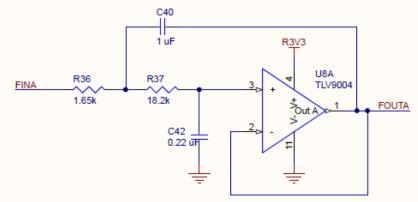
Figure 4A. One possible interface circuit for the IR sensors (option A).
