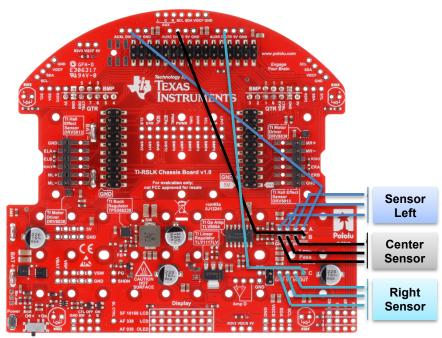
Figure 5A. Wiring up the three IR sensors with filter (option A).
