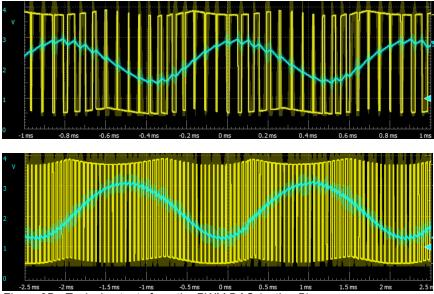
Figure 2B. Typical outputs from the PWM DAC (option B).
