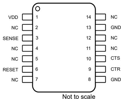
**Figure 4-1. Pin Diagram DYY Package 14-Pin SOT-23**
