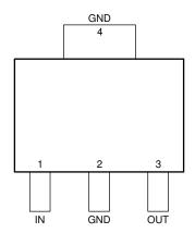
Figure 4-1. Pin Diagram (SOT-223 Package)
