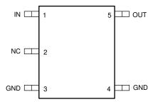
Figure 4-2. Pin Diagram (SOT-23 Package)
