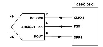
Figure 1. Hardware Interface Block Diagram
