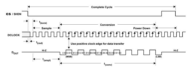
NOTE: Minimum 22 clock cycles required for 16-bit conversion. Shown are 24 clock cycles. If **CS** remains LOW at the end of conversion, a new datastream with LSB-first is shifted out again.
