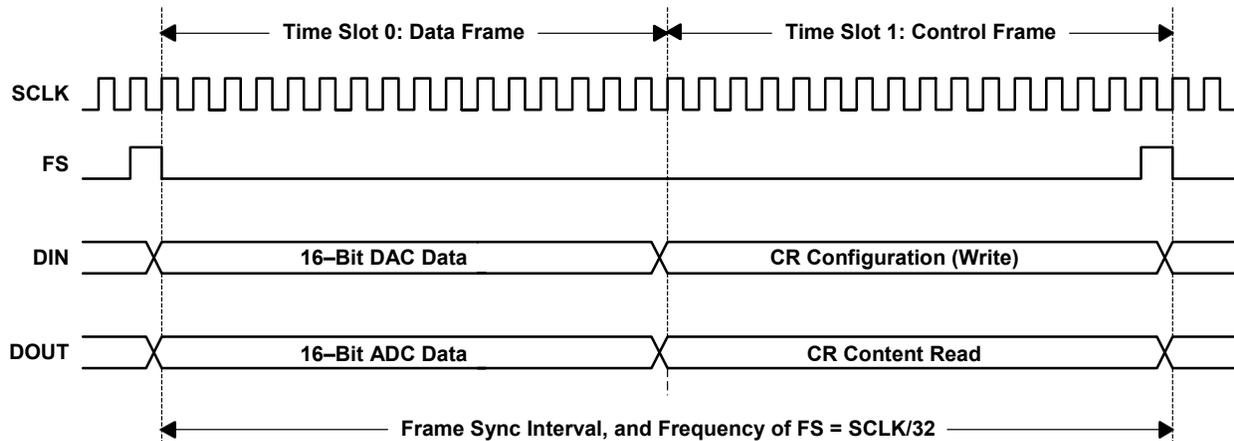
**Figure 4. Standard Programming Mode Timing, Stand-Alone Slave**
