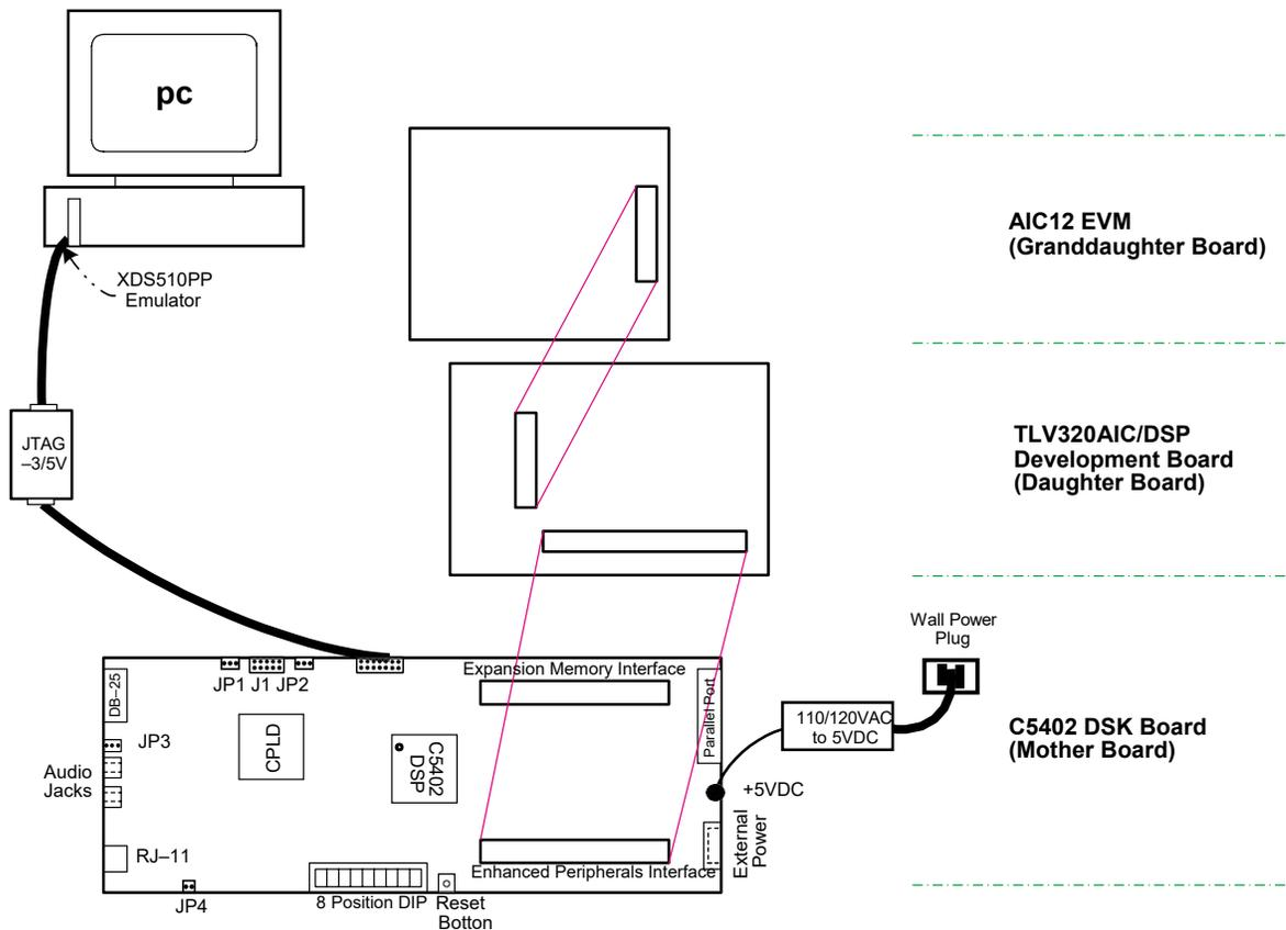
Figure 3. AIC/DSP EVM System Connection
