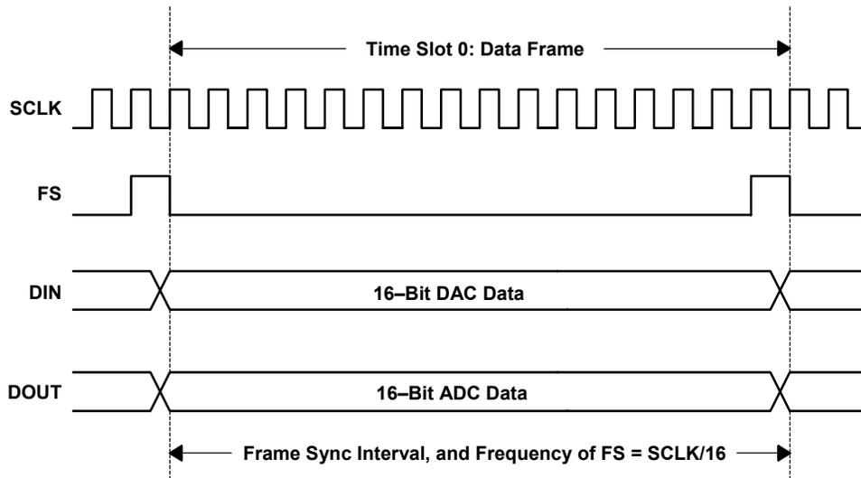
**Figure 6. Standard Continuous Mode Timing, Stand-Alone Slave**
