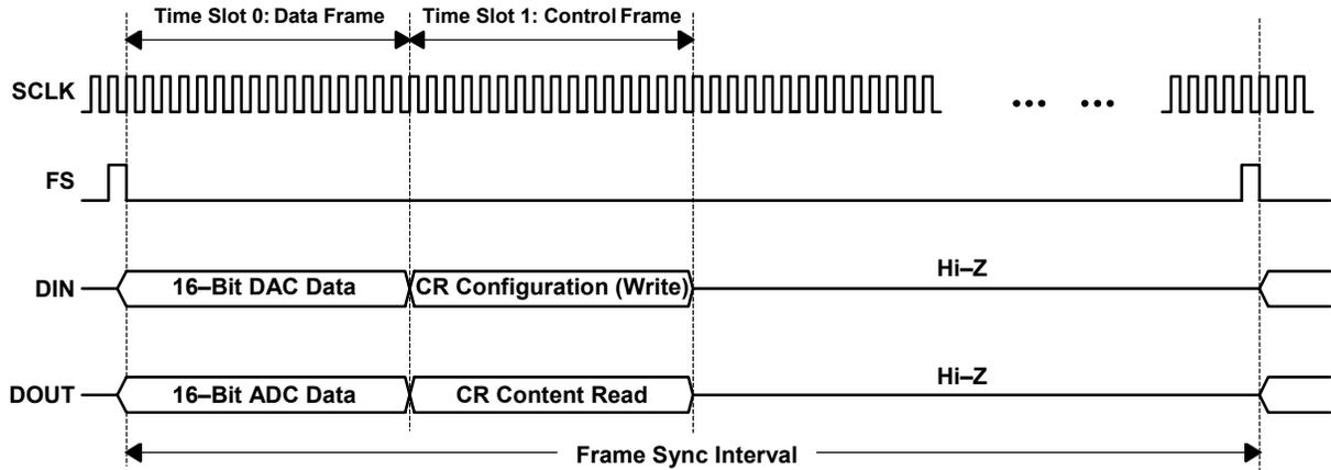
**Figure 5. Turbo Programming Mode Timing, Stand-Alone Slave**
