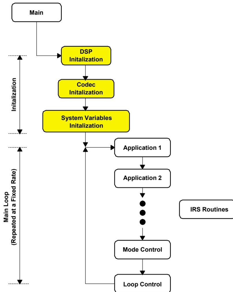
**Figure 9. DSP/Codec Firmware Structure**
