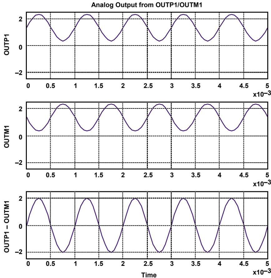
**Figure 8. Single-Ended or Differential Signals at OUTPUT1/OUTM1**
