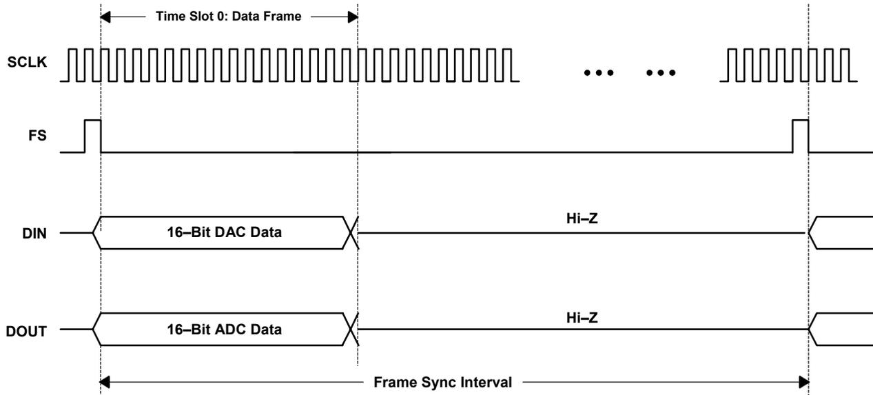
**Figure 7. Turbo Continuous Mode Timing, Stand-Alone Slave**
