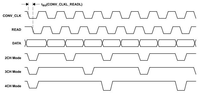
Figure 2. SYNC Pulse in 2, 3, and 4 Channel Modes
