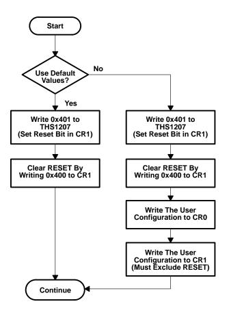
Figure 1. THS1007 Configuration Flow
