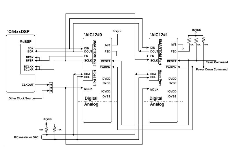
Figure 2. Typical AIC12/C54xx<sup>™</sup> DSP Digital Interface, Two-AIC12 Cascade Mode
