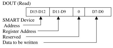
Figure 6. Control Frame Data Format
