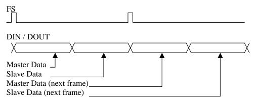
Figure 4. Master / Slave Communication in Continuous Mode
