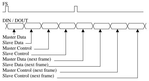
Figure 3. Master / Slave Communication in Programming Mode
