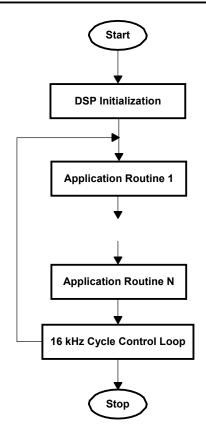
Figure 2. Main Loop Control Flow Chart
