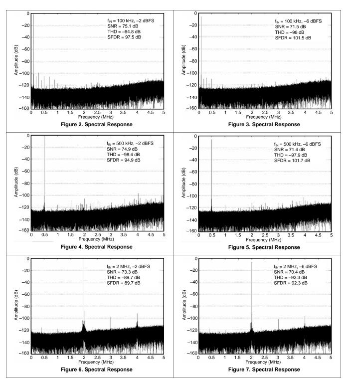
All specifications at  $T_A = 25^{\circ}$ C, AVDD = 5 V, DVDD = IOVDD = 3 V,  $f_{CLK} = 40$  MHz, External  $V_{REF} = 3$  V, 2XMODE = high,  $V_{CM} = 2$  V, and  $R_{BIAS} = 37$  k $\Omega$  (unless otherwise noted)
