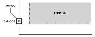
Figure 1. Pin Configuration for Doubling Output Data Rate
