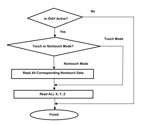
Figure 2. TSC Data Reading Sequence
