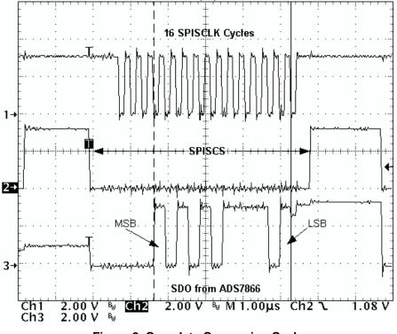
Figure 2. Complete Conversion Cycle
