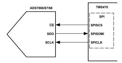
Figure 1. Hardware Interface Block Diagram
