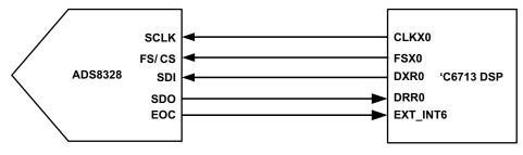
Figure 1. Hardware Connection
