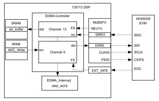
Figure 2. Data Transfer Block Diagram
