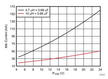
Figure 5. Idle Current vs PVDD on TAS5805M (F<sub>sw</sub> = 768 kHz, BD Mode)
