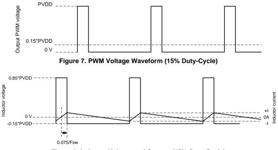
Figure 8. Inductor Voltage and Current (15% Duty-Cycle)
