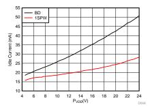
Figure 11. Idle Current vs PVDD on TAS5805M ( $F_{sw}$  = 768 kHz, 10 µH + 0.68 µF LC Filter)
