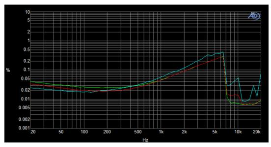
Figure 13. THD vs Input Frequency (PVDD = 12 V, Load = 6  $\Omega$ , 10  $\mu$ H + 0.68  $\mu$ F, 5-W Output Power)
