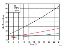
Figure 9. Idle Current vs PVDD on TAS5805M ( $F_{sw}$  = 384 kHz, 10  $\mu$ H + 0.68  $\mu$ F LC Filter)
