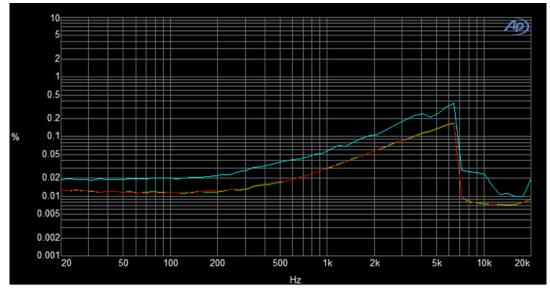
Figure 12. THD vs Input Frequency (PVDD = 12 V, Load = 6  $\Omega$ , 10 µH + 0.68 µF, 1-W Output Power)
