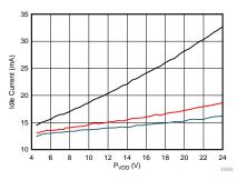
Figure 10. Idle Current vs PVDD on TAS5805M ( $F_{sw}$  = 384 kHz, 22 µH + 0.68 µF LC Filter)
