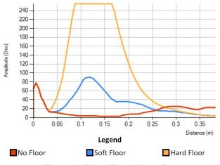
Figure 3. Floor-Type Detection
