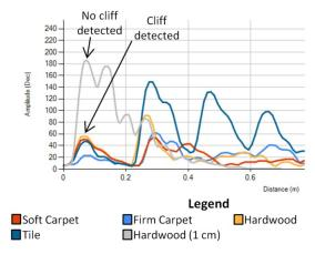
Figure 5. Cliff Detection at 20 cm
