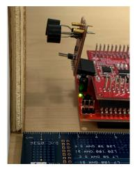
Figure 2. BOOSTXL-PGA460 Test Setup
