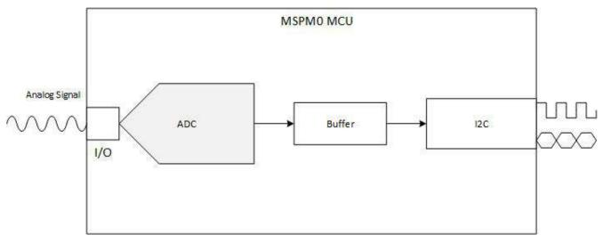
Figure 1-1. Subsystem Functional Block Diagram
