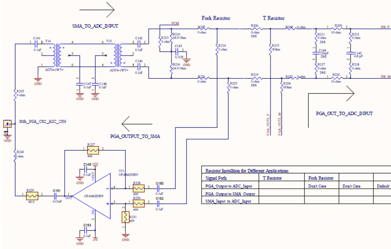
Figure 69. PGA5807 Schematic, (Sh. 7 of 16), PGA\_CH2, ADC\_CH6
