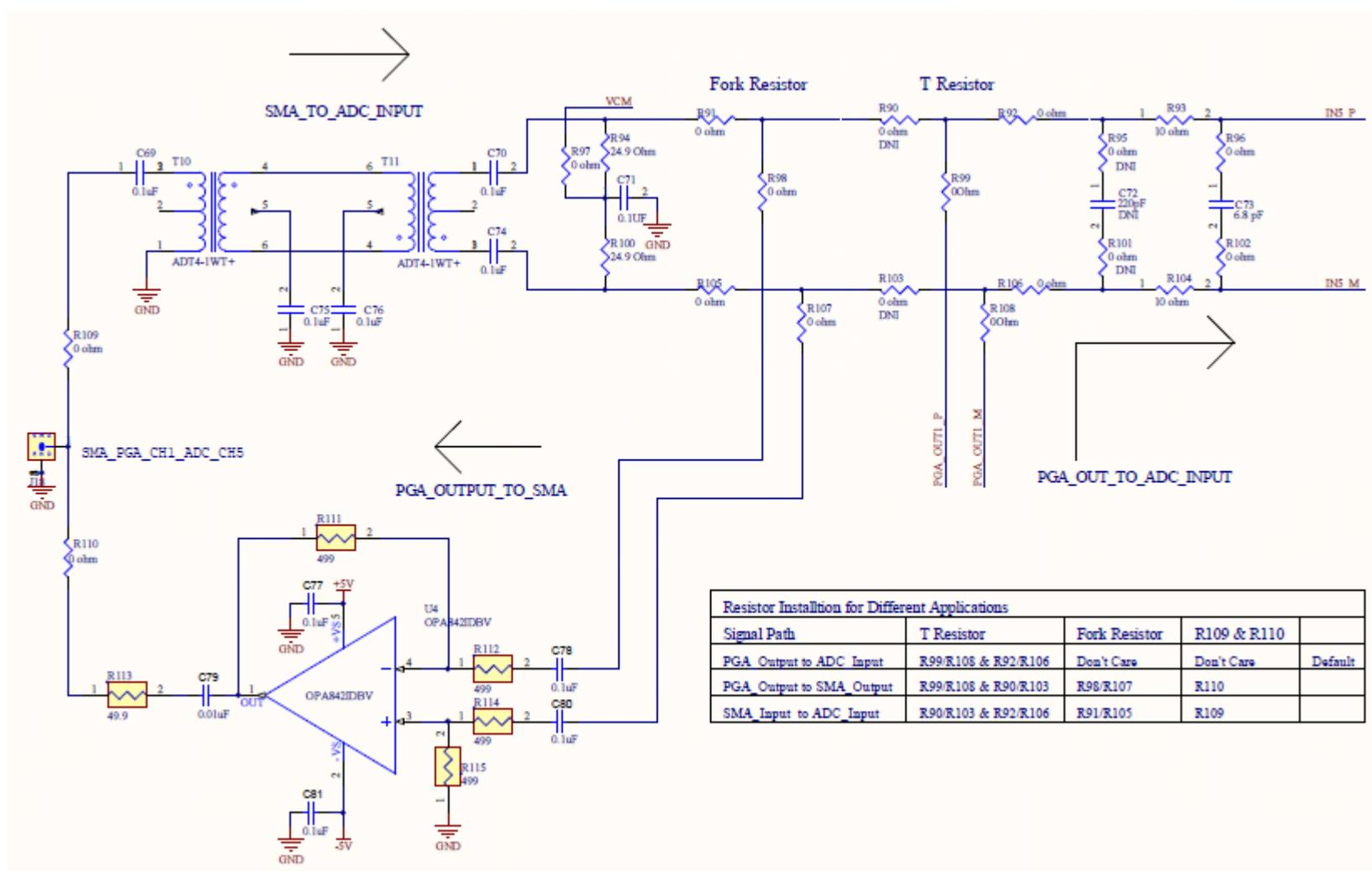
Figure 68. PGA5807 Schematic, (Sh. 6 of 16), PGA\_CH1, ADC\_CH5
