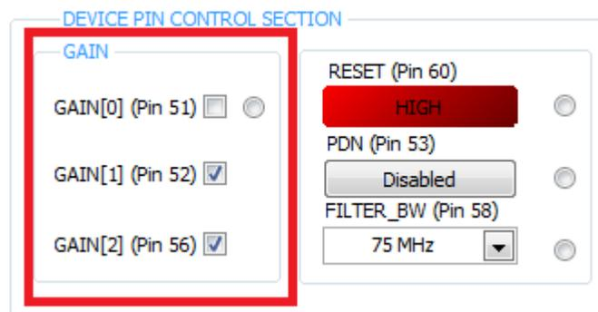
Figure 50. PGA5807 GUI Setup for PGA5807+ADS5296 Gain Test 4
