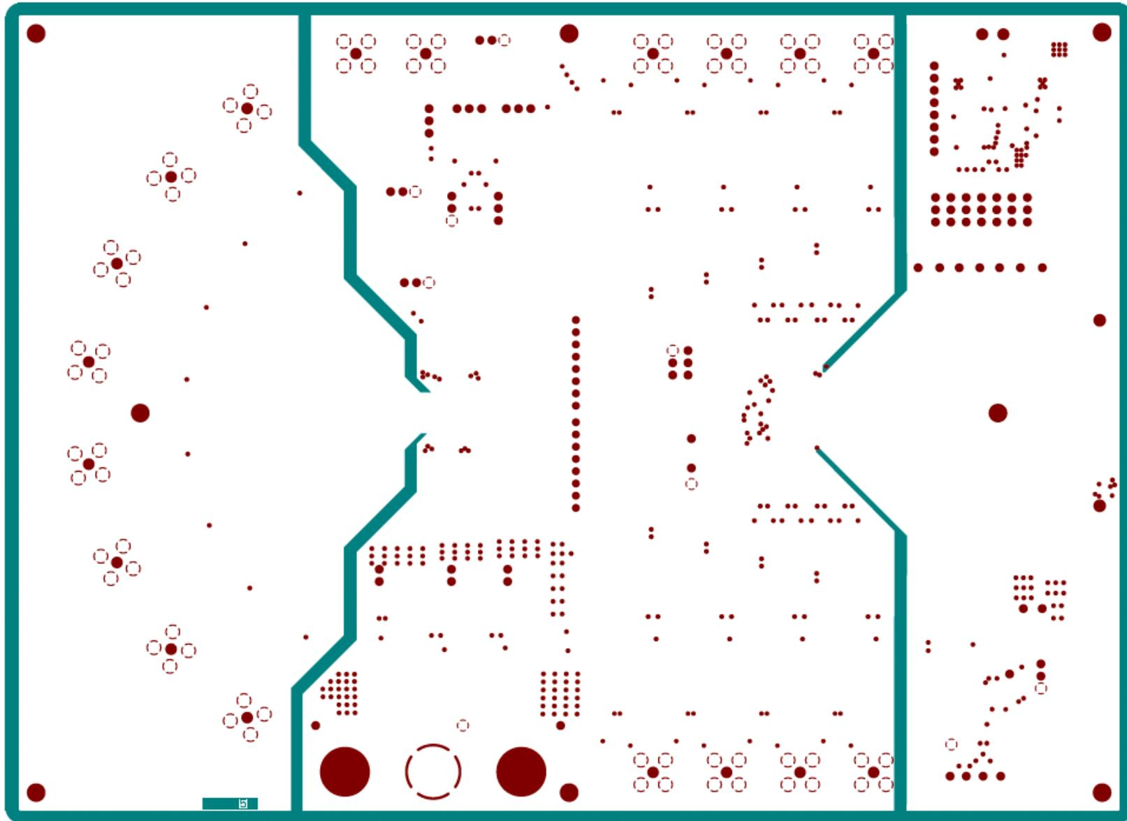
Figure 85. PGA5807 EVM GND Split Plane 2
