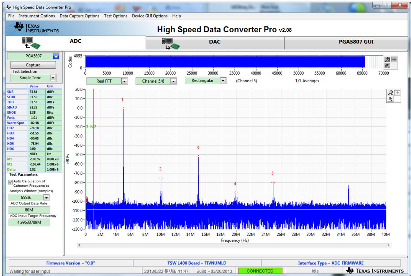
Figure 45. PGA5807+ADS5296 SNR, THD, Gain Test Capture 1
