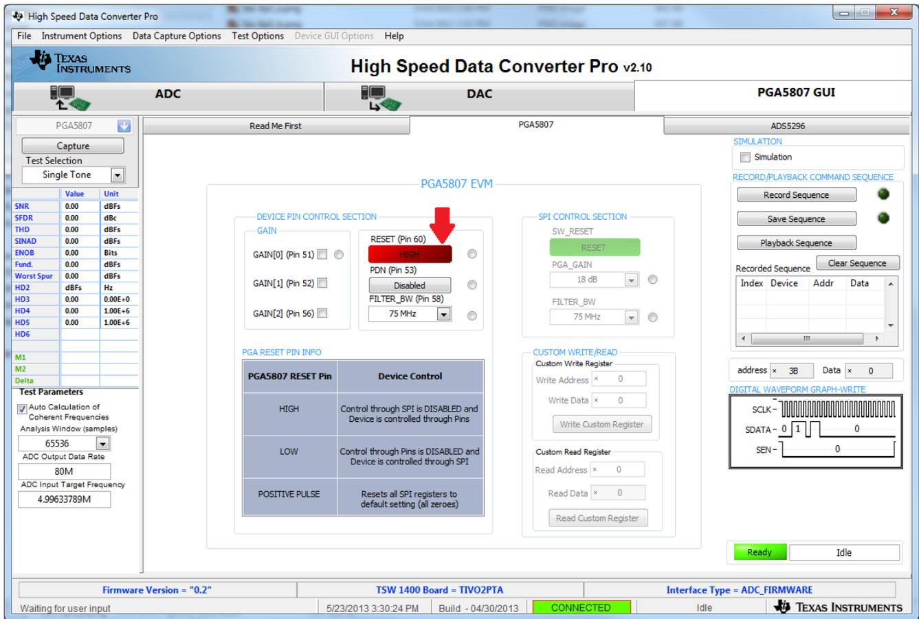
Figure 48. PGA5807 GUI Setup for PGA5807+ADS5296 Gain Test 3
