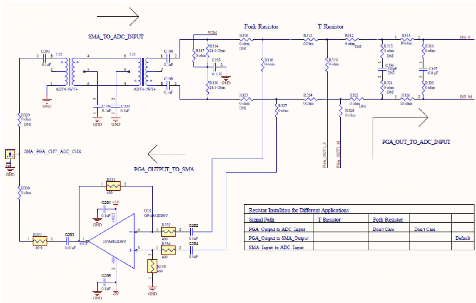
Figure 74. PGA5807 Schematic, (Sh. 12 of 16), PGA\_CH7, ADC\_CH3
