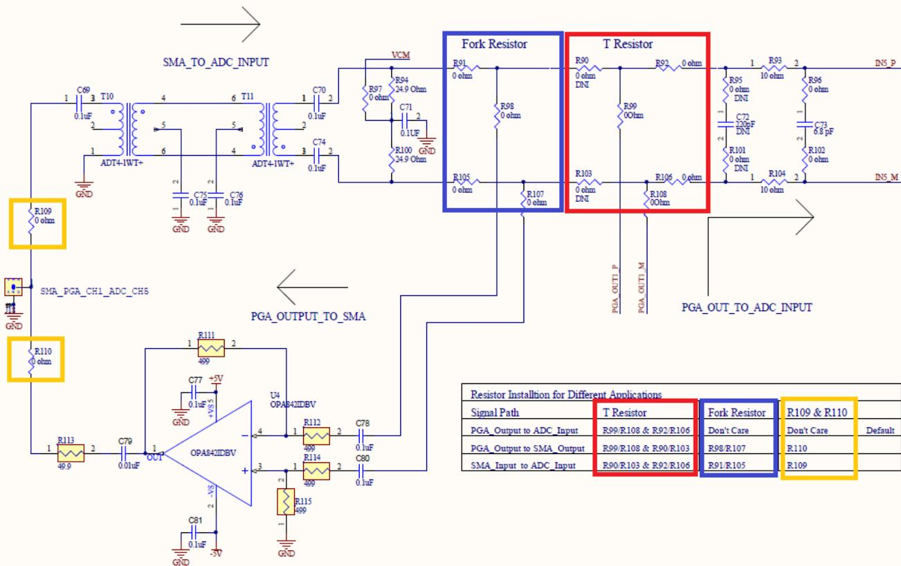
Figure 21. PGA5807 EVM Schematic 0-Ω JUMper Options
