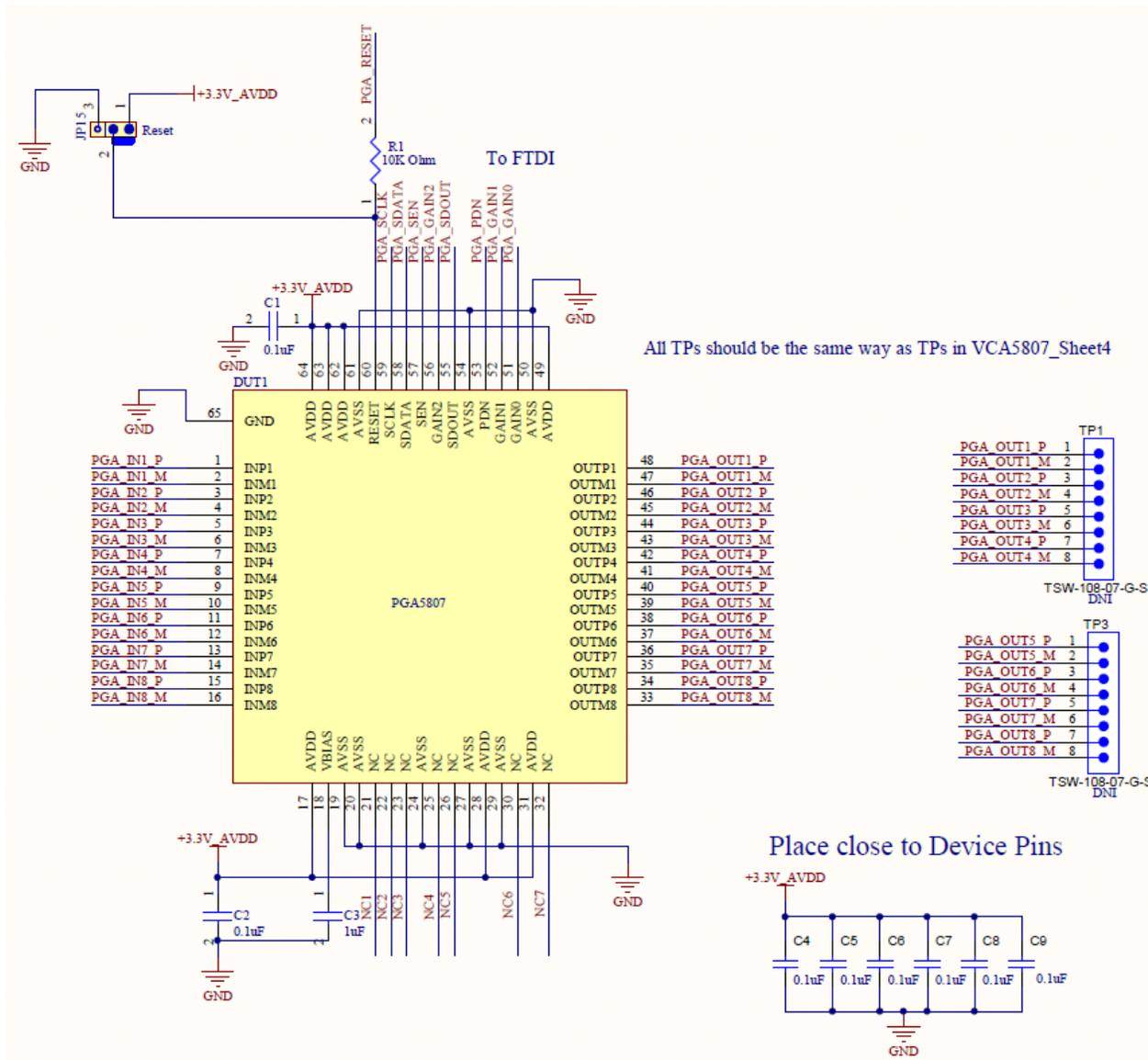
Figure 63. PGA5807 Schematic, (Sh. 1 of 16), PGA5807 Device
