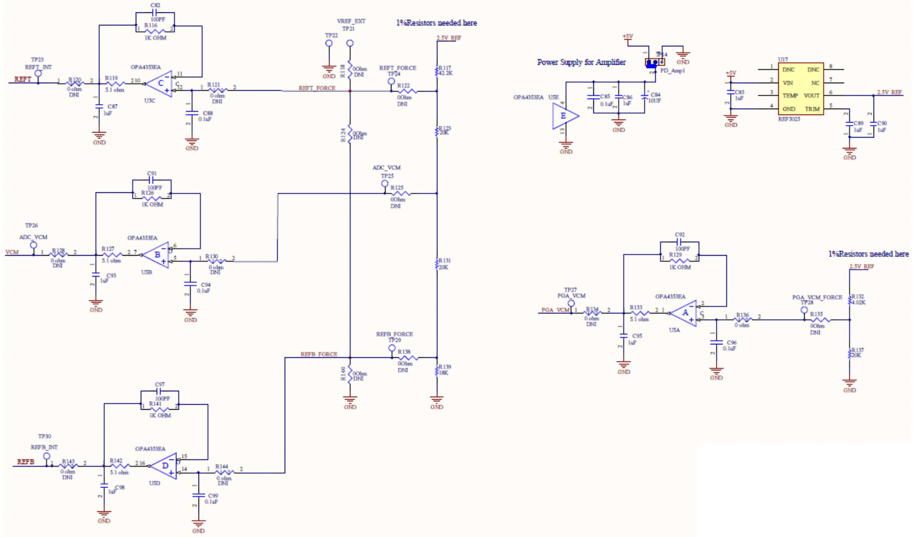
Figure 77. PGA5807 Schematic, (Sh. 15 of 16), ADS5296 External Reference
