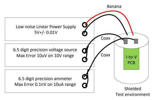
Figure 12: Test Setup for V-to-I Board
