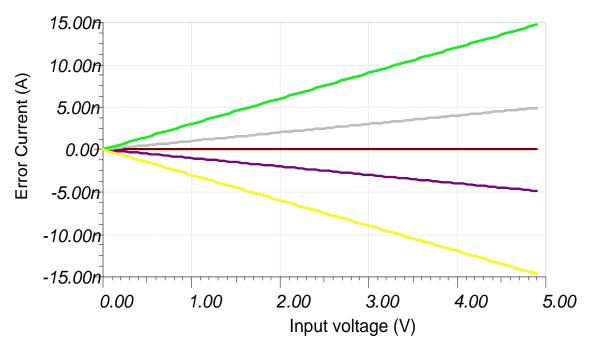
Figure 10: Monte Carlo Analysis for Resistor Tolerance
