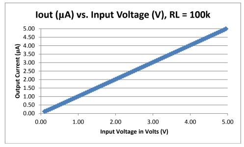
Figure 13:  $I_{OUT}$  vs.  $V_{IN}$  for 100 k $\Omega$  Load
