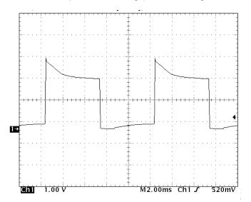
Figure 18: Large signal at bandwidth limit (100 Hz)
