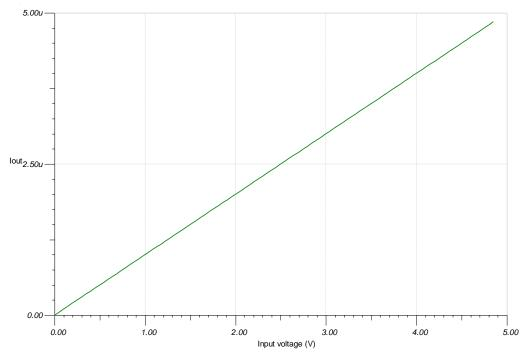
Figure 6: Simulation DC Transfer Results (RL = 500 k $\Omega$ )
