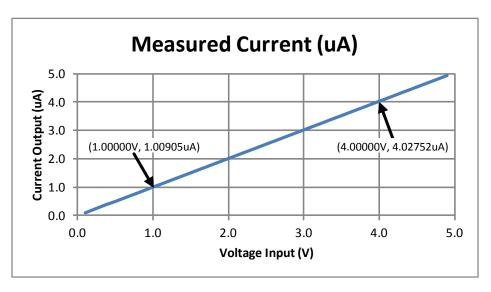
Figure 15: Measured current showing two points used in calibration
