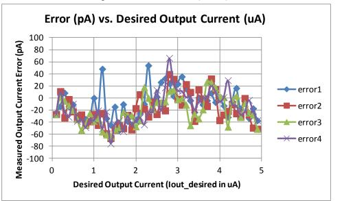
Figure 16: Measured output error post calibration for 0.1  $\mu$ A < I<sub>out</sub> < 4.9  $\mu$ A
