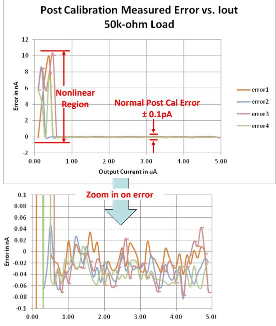
Figure 22: Post calibration error showing nonlinearity error for low op amp outputs
