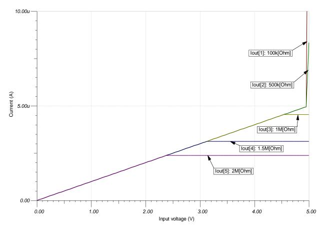
Figure 9: Compliance Voltage vs. Load Resistance Simulation
