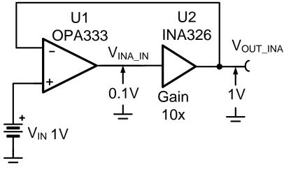
Figure 3: Simplified Composite Amplifier
