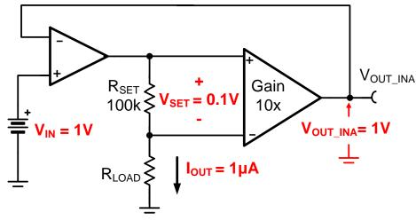
Figure 4: Simplified I-to-V
