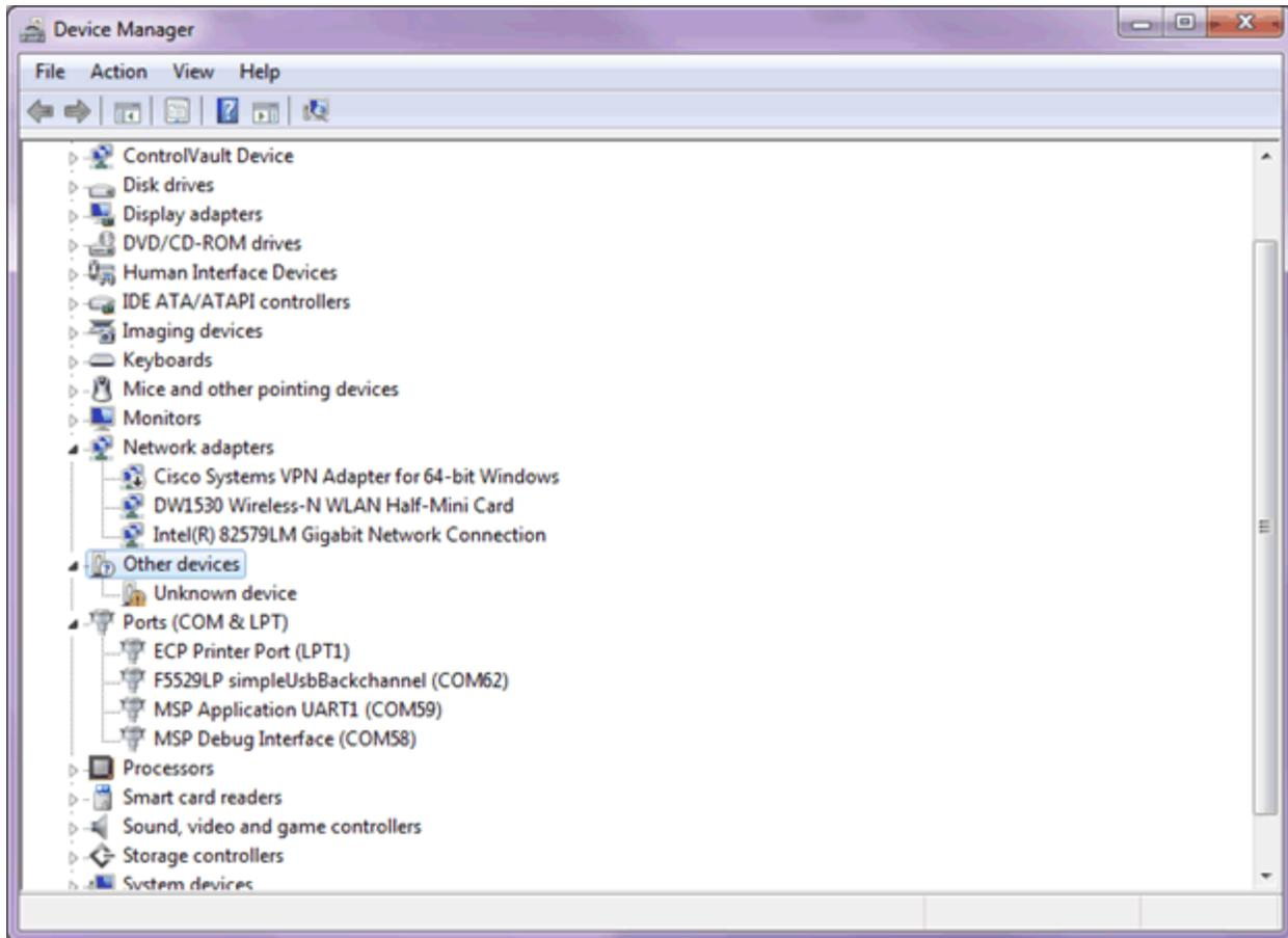
**Figure 33. Device Manager After Both Ports are Enumerated**
