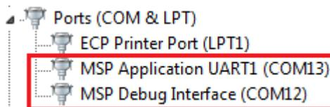
**Figure 15. Application Backchannel UART in Device Manager**
