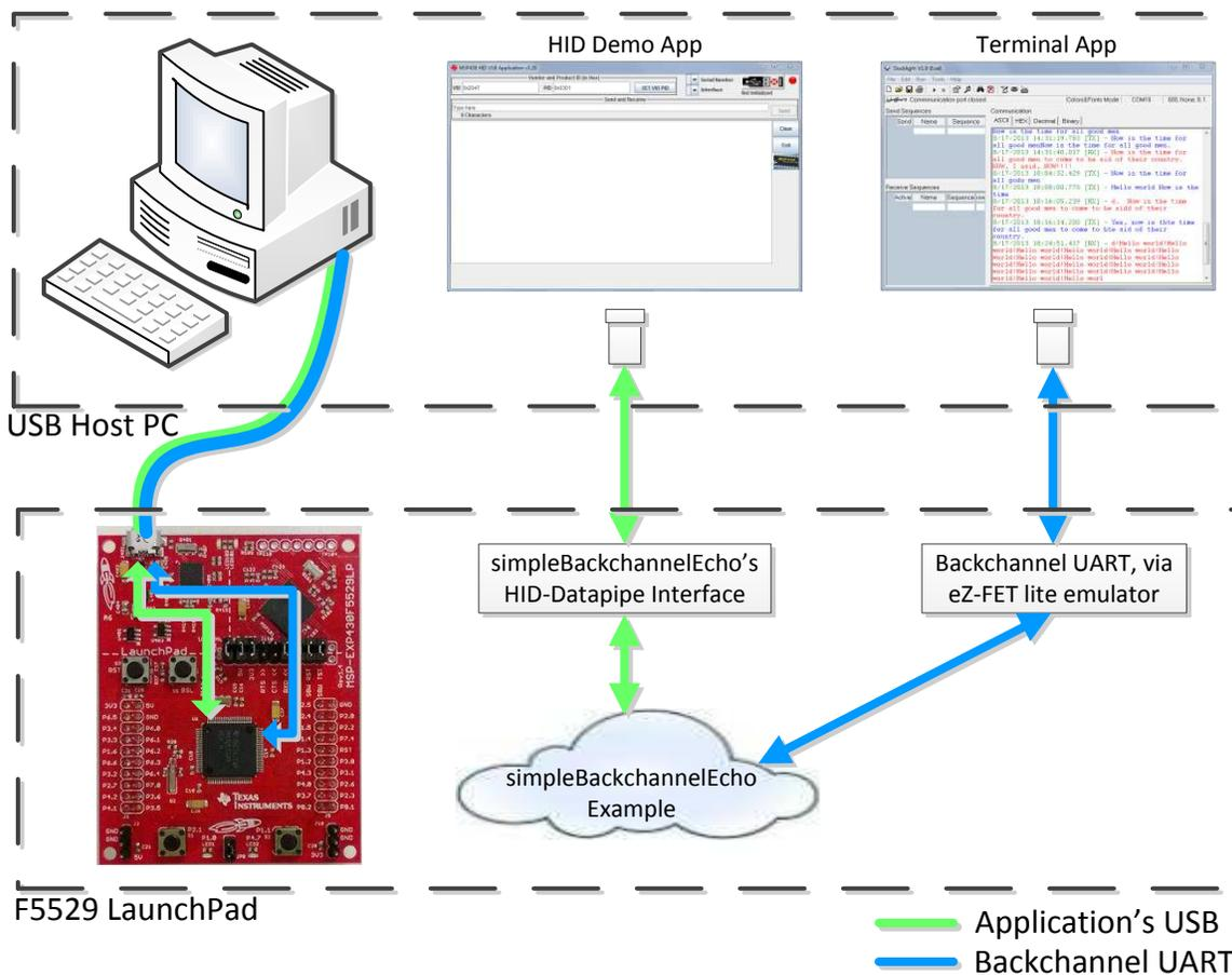
Figure 34. Movement of Data in simpleUsbBackchannel: HID-Datapipe
