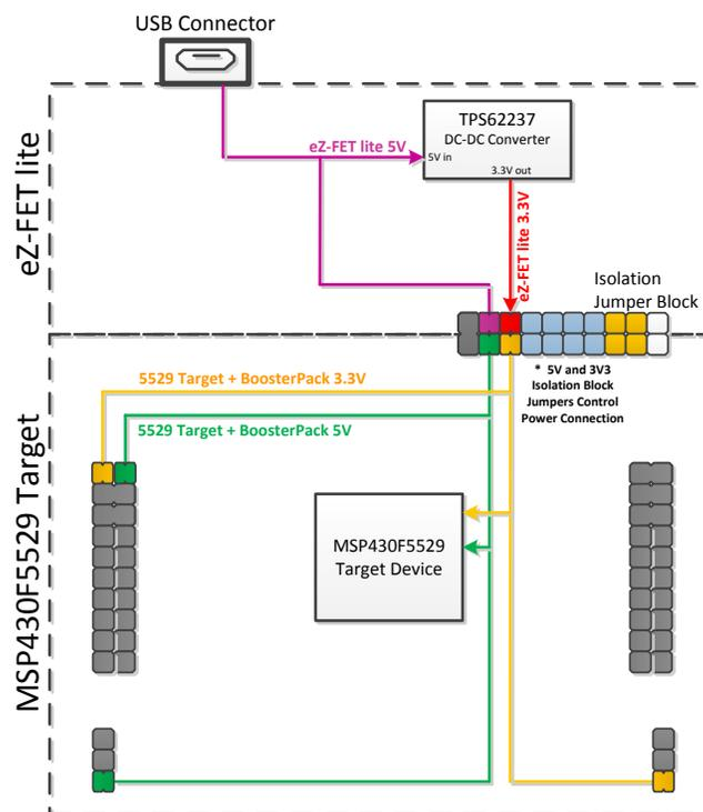
**Figure 13. F5529 LaunchPad Development Kit Power Supply**
