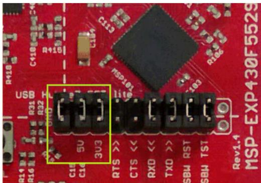
**Figure 2. Jumper Requirements Necessary for Software Demo**
