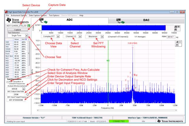
Figure 7. High Speed Data Converter Pro (HSDC) GUI
