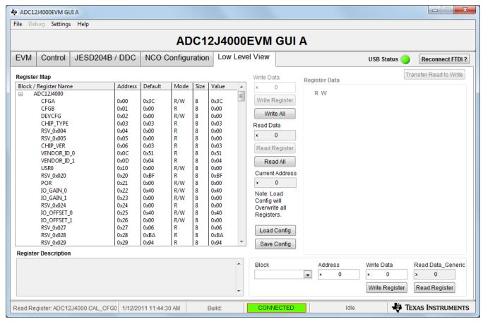
Figure 9. Low-Level Register Control Tab
