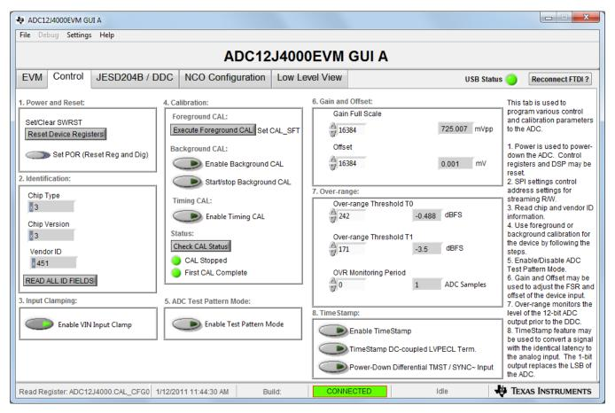
Figure 6. Configuration GUI ADC Control
