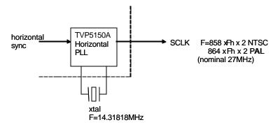
Figure 9. Line-Locked Sampling
