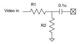
Figure 2. TVP5150A Input Termination
