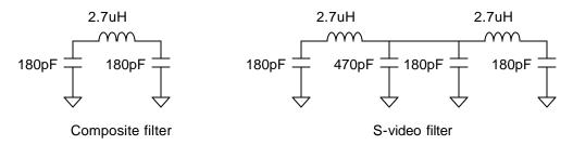
Figure 3. Example Anti-Alias Filters for Composite and S-Video
