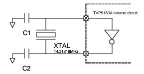
Figure 5. TVP5150A Crystal Circuit
