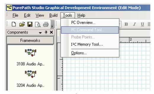
Figure 2-2. Setting the I<sup>2</sup>C Initialization Sequence
