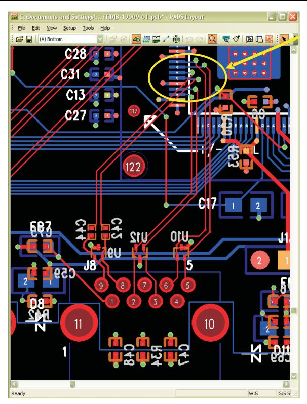
Figure 1. Using Via Placement to Cross the SSTX and SSRX Pairs
