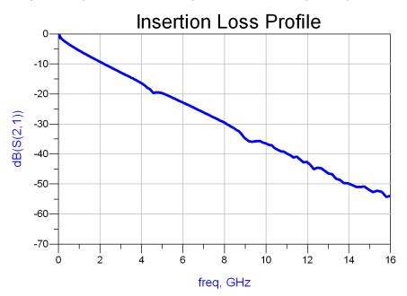
Figure 1. Insertion Loss (SDD21) – 24in x 4mil Trace
